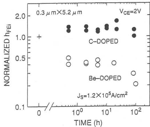
Fig. 4. Dependence of  $h_{FEi}$  on the stress duration. The stress current density was kept at a constant value of  $1.2 \times 10^5 A/cm^2$ .
