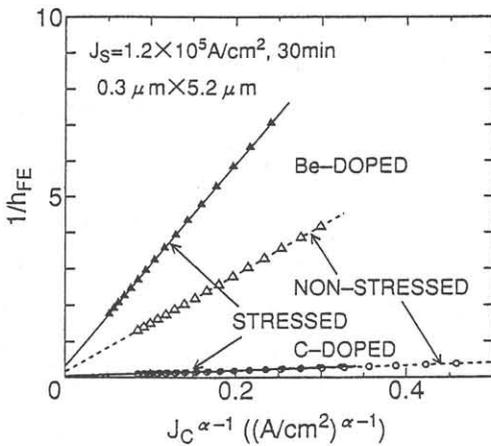
Fig. 2. Plots of  $1/h_{FE}$  as a function of  $J_C^{\alpha-1}$ . Current gain  $h_{FE}$  measured is described as  $1/h_{FE} = 1/h_{FEi} + K J_C^{\alpha-1}$ , where  $h_{FEi}$  is the intrinsic current gain and obtained from the intercept with the y-axis.
