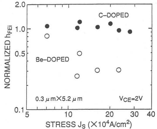
Fig. 3. Dependence of  $h_{FEi}$  on the stress current density  $J_s$ . The ordinate indicates the ratio of  $h_{FEi}$  after the forward-bias test to the initial value.
