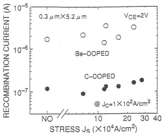
Fig. 5. Dependence of the recombination current on  $J_s$ .
