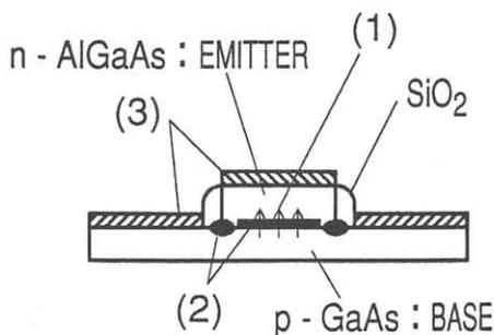
Fig. 1. Degradation factors: 1) the base-dopant diffusion, 2) the change in recombination current, and 3) the degradation of ohmic resistances.
