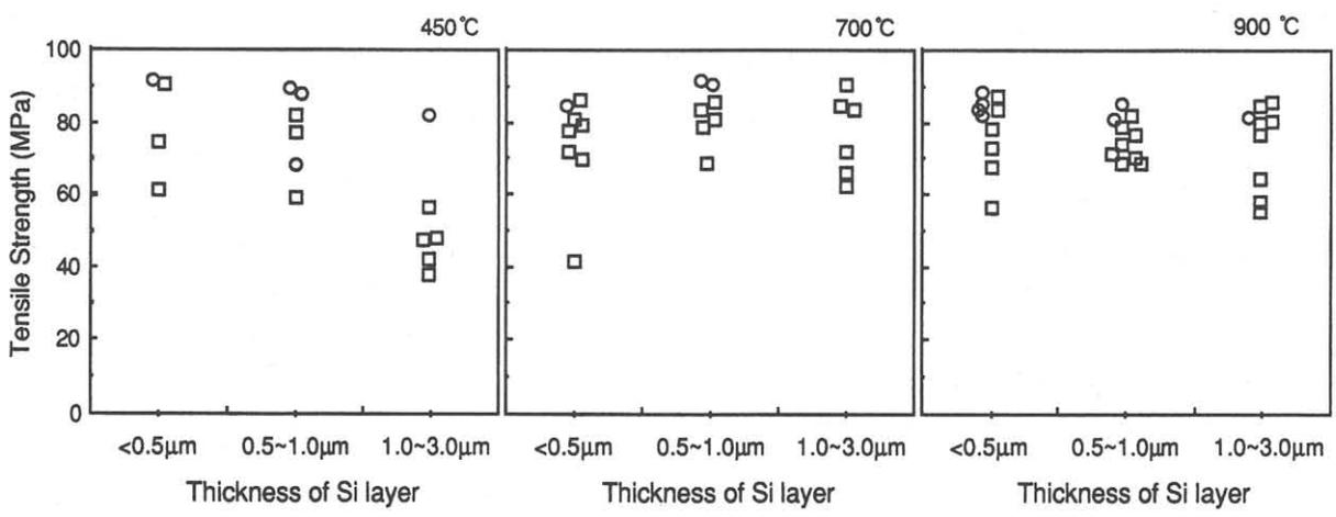
Fig. 3 Thickness dependence of tensile strength of bonded silicon - sapphire samples on various temperatures.
