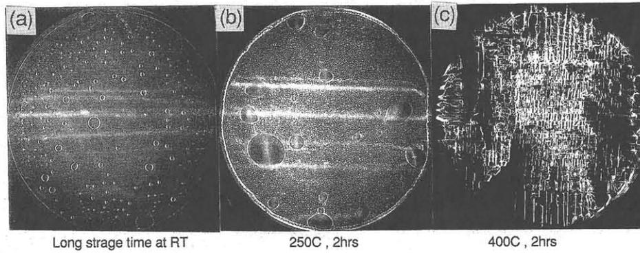
Fig. 1 X - ray topographs of bonded silicon - sapphire wafers (4 inch diameter). Voids generated by long storage time at RT (a), voids generated by annealed by annealing at 250 C without crack. Large voids induced by particles (b), and cracks in silicon at 400 C for 2 hrs in dry O<sub>2</sub> (c).
