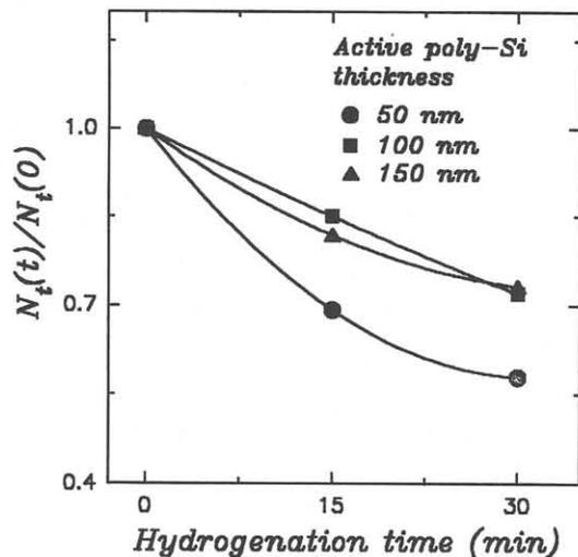
Fig. 4. Normalized variation of trap state density with hydrogenation time for various active poly-Si thickness ( $50, 100$  and  $150 \text{ nm}$ ). The symbol  $t$  refers to hydrogenation time.
