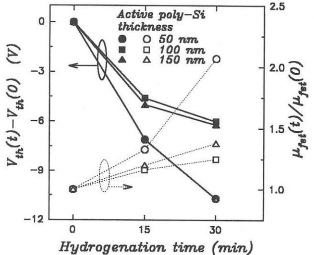
Fig. 3. Threshold voltage shift ( $\Delta V_{th} = V_{th}(t) - V_{th}(0)$ ) and normalized increment of field effect mobility ( $\mu_{fet}(t)/\mu_{fet}(0)$ ) as a function of hydrogenation time for various active poly-Si thickness. Gate poly-Si thickness of N-channel poly-Si TFT's was  $100 \text{ nm}$  and  $W/L = 20/10 \mu\text{m}/\mu\text{m}$ . The symbol  $t$  refers to hydrogenation time.
