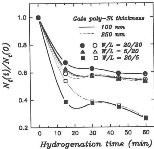
Fig. 6. Normalized variation of trap state density with hydrogenation time for different gate poly-Si thickness and various channel dimensions. The symbol  $t$  refers to hydrogenation time.
