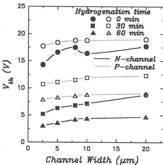
Fig. 2. Variation of threshold voltage as a function of channel width for  $L = 20 \mu\text{m}$  N- and P-channel poly-Si TFT's with different hydrogenation time. The thickness of gate and active poly-Si is  $100 \text{ nm}$ .
