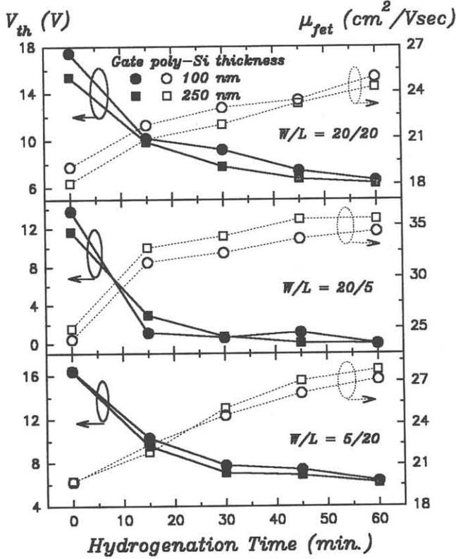
Fig. 5. Threshold voltage ( $V_{th}$ ) and field effect mobility ( $\mu_{fet}$ ) as a function of hydrogenation time for N-channel poly-Si TFT's with different gate poly-Si thickness and various channel dimensions.
