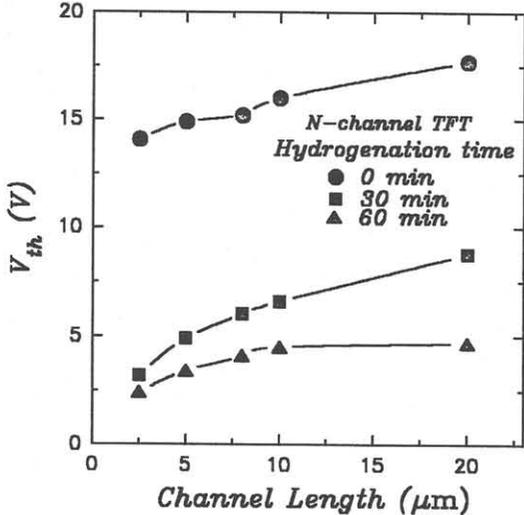
Fig. 1. Variation of threshold voltage as a function of channel length for  $W = 20 \mu\text{m}$  N- and P-channel poly-Si TFT's with different hydrogenation time. The thickness of gate and active poly-Si is  $100 \text{ nm}$ .
