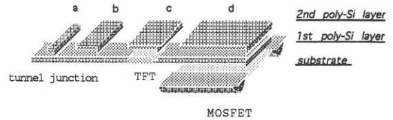
Figure 2: Structure of the fabricated new analog memory. a: tunnel gate, b: bias gate, c: TFT gate, and d: control gate.
