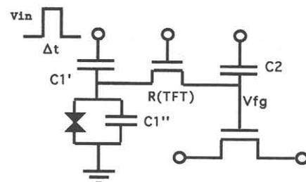
Figure 1: Equivalent circuit of the new analog memory.
