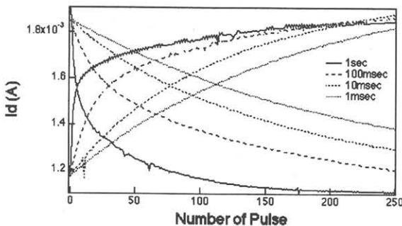
Figure 6: Experimental result of the drain current as a function of the number of input pulses (injection/extraction) for four values of the pulse widths.
