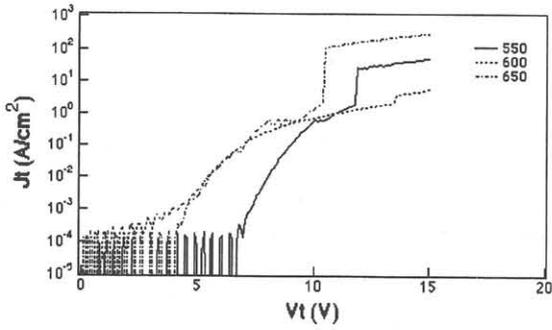
Figure 4: I-V characteristics of the tunnel junctions (the oxide thicknesses are 200Å) which have been fabricated in the deposition of SiH<sub>4</sub> at 600°C and 650°C, Si<sub>2</sub>H<sub>6</sub> at 550°C.
