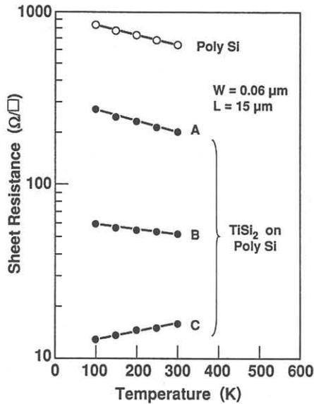
Figure 5: Temperature dependence of sheet resistance of  $0.06 \mu\text{m}$  wide,  $15 \mu\text{m}$  long  $\text{TiSi}_2$  gates. A, B, C denote samples having various resistances shown in Fig.4. A and B exhibited semiconductor-like behavior, whereas, C exhibited metallic behavior.
