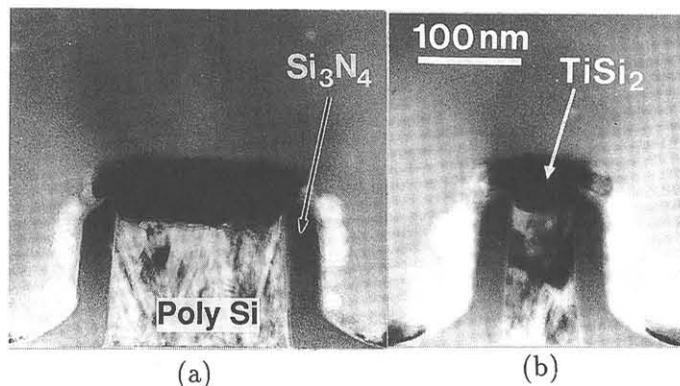
Figure 1: Cross-sectional TEM view of  $\text{TiSi}_2$  gate for (a) 0.17  $\mu\text{m}$  width and (b) 0.06  $\mu\text{m}$  width gate.
