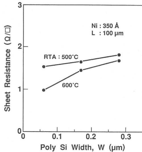
Figure 7: Poly Si width dependence of sheet resistance in NiSi gate for two silicidation temperatures. The sheet resistance is mostly independent of poly Si width or rather decreased as the line width decreased to less than  $0.1 \mu\text{m}$ .
