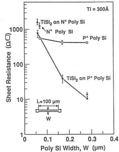
Figure 3: Poly Si width (W) dependence of sheet resistance for TiSi<sub>2</sub> silicided gate (●,▲) and non-silicided gate (○,◻). A significant increase in sheet resistance is observed with a silicided 0.06 μm poly Si gate.
