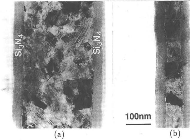
Figure 2: Planar TEM view of TiSi<sub>2</sub> gate for (a) 0.28 μm width and (b) 0.06 μm width gate.
