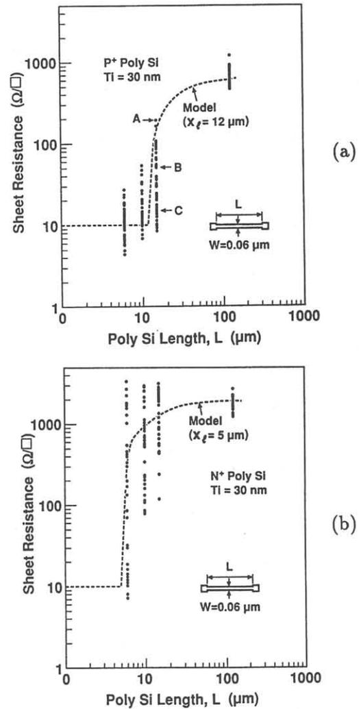
Figure 4: Poly Si line length (L) dependence of sheet resistance in 0.06 μm width TiSi<sub>2</sub> gate for (a) P<sup>+</sup> and (b) N<sup>+</sup> poly Si gates. The sheet resistance increased significantly with an increase in poly Si length, for both cases.
