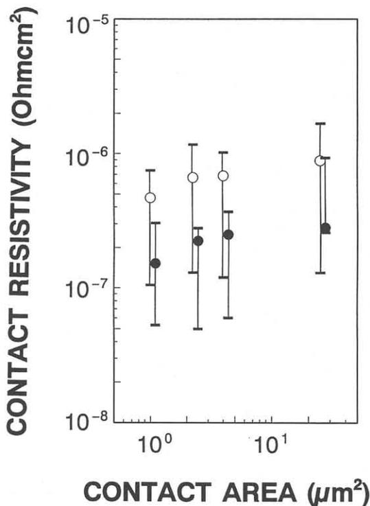
Fig.5 Dependence of W/n<sup>+</sup>-Si contact resistance on the pre-treatment process. The symbols ○ and ● represent conventional and N<sub>2</sub> sealed processes, respectively.
