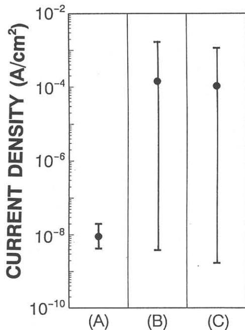
Fig.3 Dependence of reverse leakage current of  $W/n^+p$  junction on conditions of initial tungsten growth, (A)  $WF_6/SiH_4=10/0$ SCCM, (B)  $WF_6/SiH_4=10/0.5$ SCCM, and (C) no additional step.
