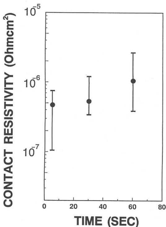
Fig.4 Dependence of W/n<sup>+</sup>-Si contact resistance on initial film formation time.
