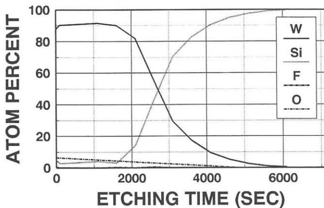
Fig.2 XPS depth profiles of W, F, O, and Si in a tungsten film.
