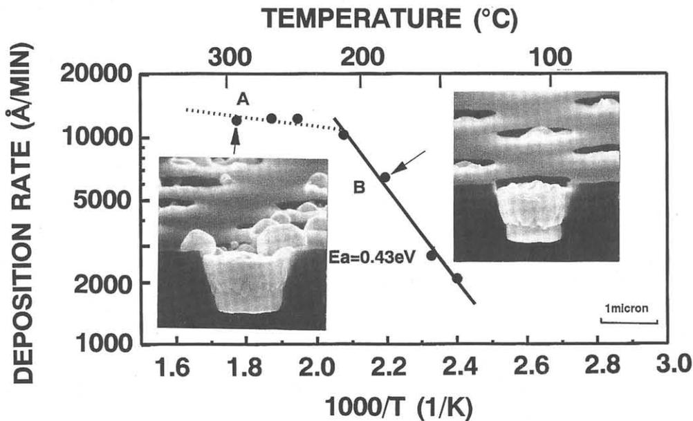
Fig.1 Arrhenius plot of tungsten deposition rate, where  $WF_6/SiH_4/H_2/Ar=10/4/100/100$  SCCM and  $P_T=138mTorr$
