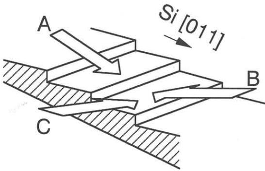
Fig. 2 Three different Al incidence configurations with respect to the ideal atomic step of the misoriented (100)Si surface tilted toward the [011] direction.
