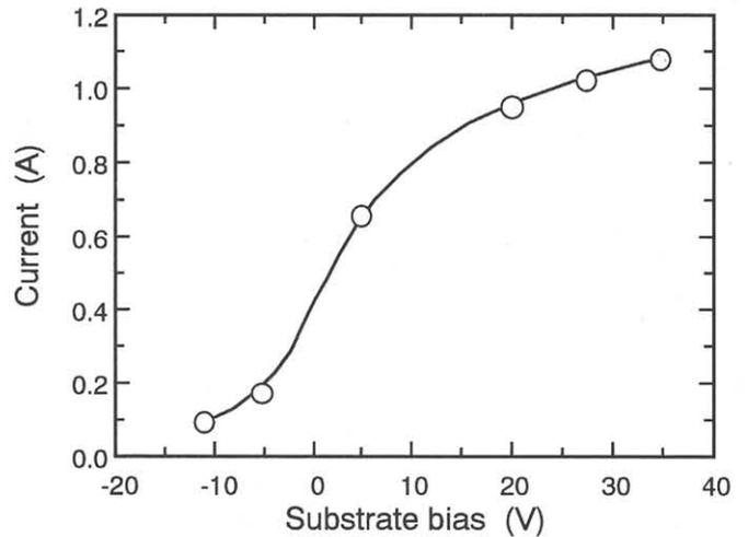
Fig. 5 I-V characteristics of Ar plasma measured at substrate electrode. Target voltage is -500V, Ar pressure is  $9 \times 10^{-4}$  Torr. Admission of hydrogen gas does not significantly affect the I-V curve.
