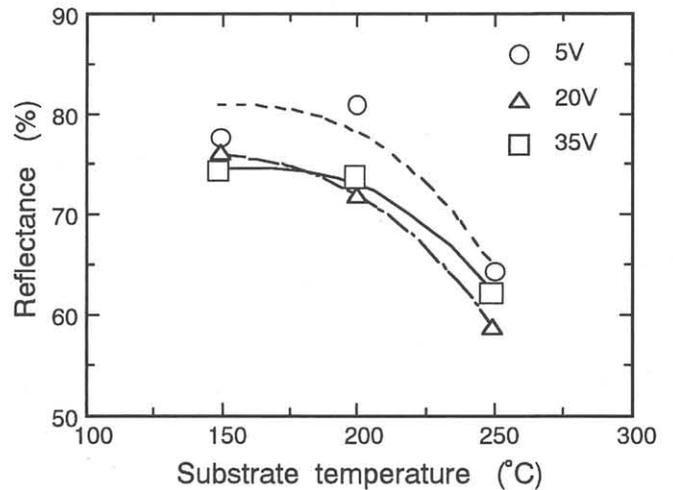
Fig. 4 Substrate temperature dependence of the optical (He-Ne laser) reflectance of Al.
