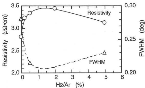
Fig. 7 Hydrogen content dependence of the resistivity and FWHM of Al(220) peak. The resistivity was measured for the polycrystal film deposited on SiO<sub>2</sub> at zero bias at 400°C, and the FWHM was measured for the single crystal Al(110) grown at a bias of +5V at 250°C.
