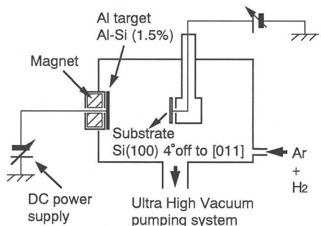
Fig. 1 Schematic diagram of UHV dc magnetron sputtering machine, in which hydrogen gas can be admitted and substrate bias can be applied. The ultimate pressure is  $5 \times 10^{-10}$  Torr utilizing 1500l/s cryo pump.
