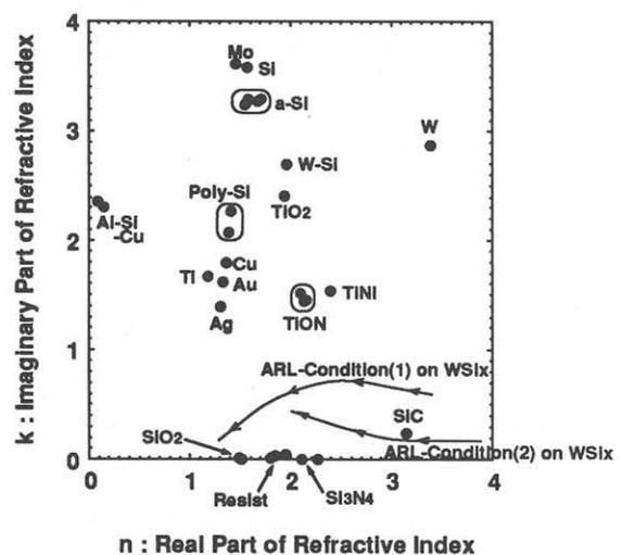
Fig. 1 Refractive indices of Various materials at 248nm. Plotted curves are simulated anti-reflective n and k values on WSix.
