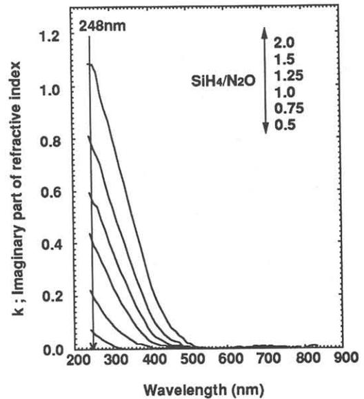
Fig. 3 Wavelength dependence on imaginary part of refractive index (k).
