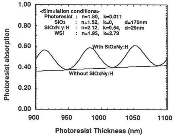
Fig. 6 Simulated photoresist absorption with and without SiOxNy:H for WSix substrate.
