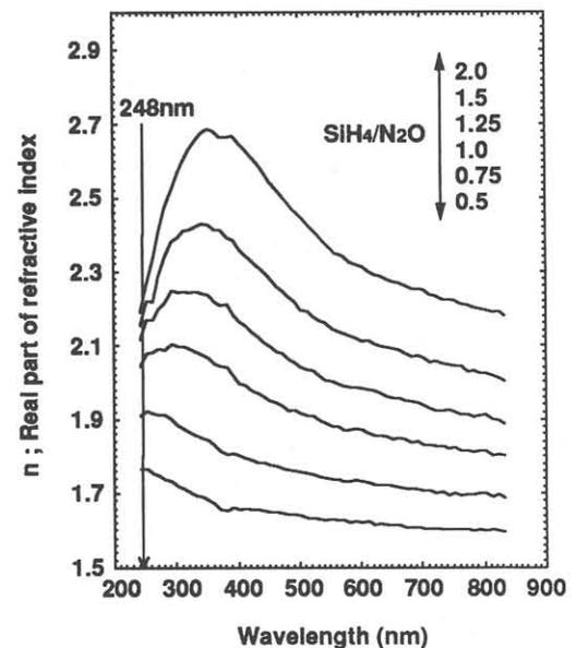
Fig. 4 Wavelength dependence on real part of refractive index (n).
