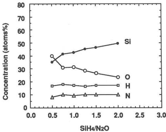
Fig. 5 SiH<sub>4</sub>/N<sub>2</sub>O ratio dependence on concentration of Si, O, H and N.
