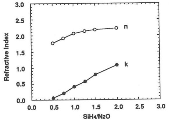
Fig. 2  $\text{SiH}_4/\text{N}_2\text{O}$  ratio dependence of n and k at 248nm.
