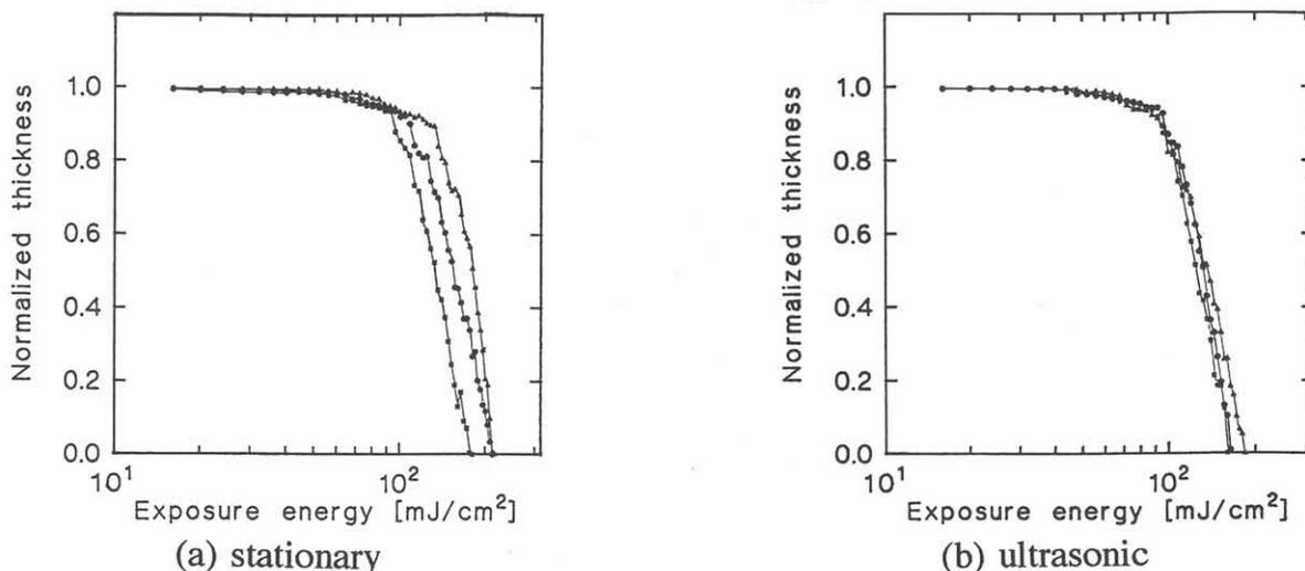
**Figure 1.** Contrast curves of resist developed by means of (a) stationary and (b) ultrasonic developing under the same conditions.
