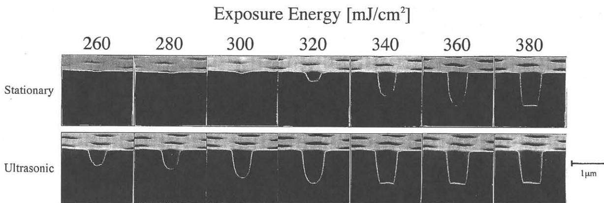
**Figure 3.**  $0.6\mu\text{m}$  contact hole patterns developed with and without ultrasonic waves as a function of exposure energy. A g-line stepper was employed. The focus was  $+0.5\mu\text{m}$ .
