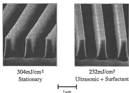
**Figure 6.**  $0.6\mu\text{m}$  line-and-space patterns by using ultrasonic developing with surfactant.
