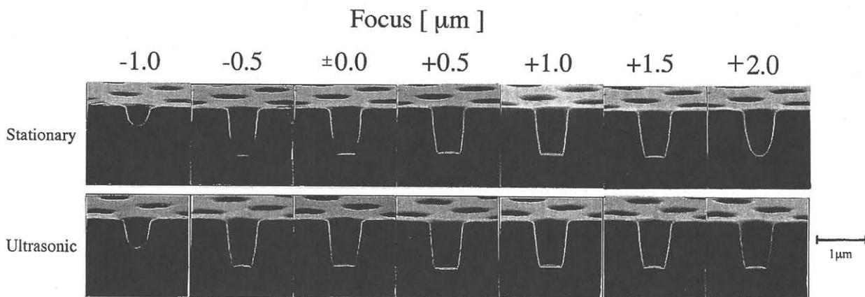
**Figure 4.** Defocus characteristics of  $0.6\mu\text{m}$  contact hole patterns developed with and without ultrasonic waves at an exposure energy of  $380\text{ mJ/cm}^2$  and  $360\text{ mJ/cm}^2$ , respectively. A g-line stepper was employed.
