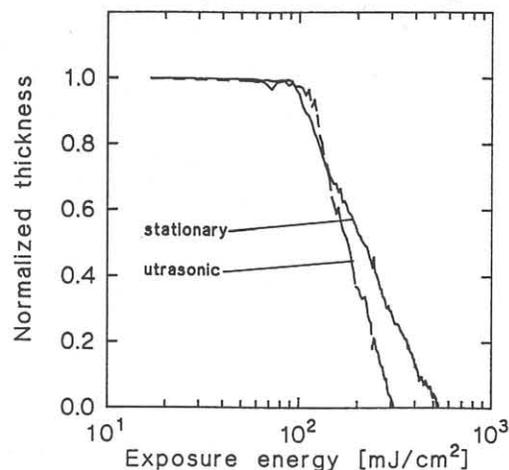
**Figure 2.** Contrast curves of the thick-film resist developed with and without ultrasonic waves. The resist thickness was  $2.7\mu\text{m}$ .
