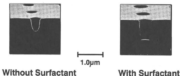
**Figure 5.**  $0.3\mu\text{m}$  contact hole patterns formed by the developer with and without surfactant and an i-line stepper ( $410\text{mJ/cm}^2$ ).
