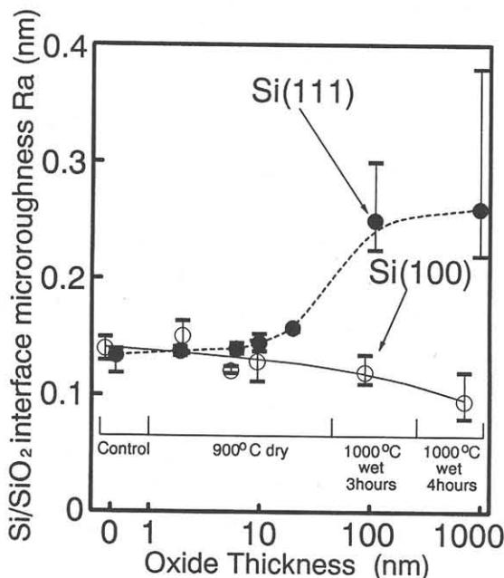
**Figure 1.** The relationship between Si-SiO<sub>2</sub> interface microroughness and oxide thickness.
