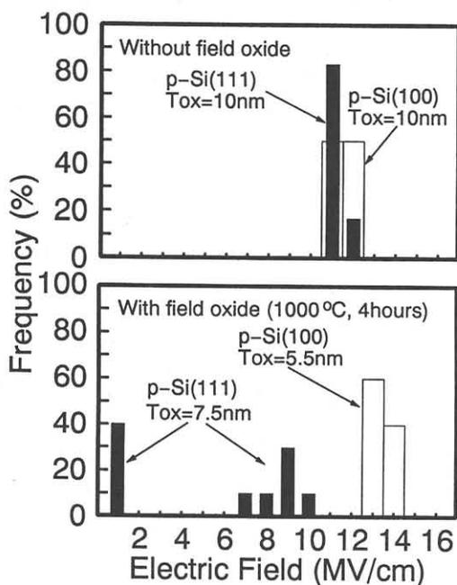
**Figure 2.** The dielectric breakdown histogram for Si(100) and Si(111).
