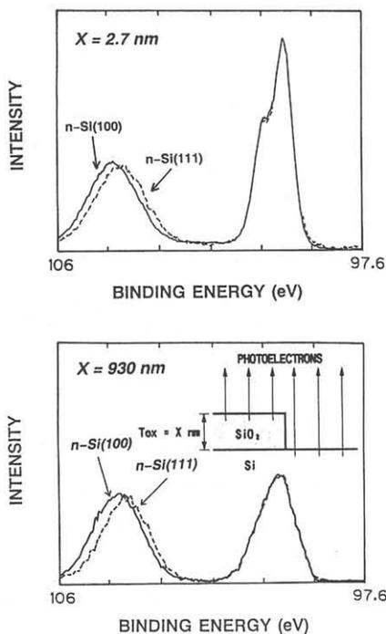
**Figure 5.** The  $Si_{2p}$  XPS spectra for the oxides on Si(100) and Si(111).
