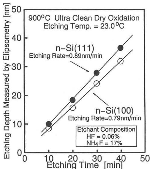
**Figure 4.** Etching depth of oxide films as a function of etching time.
