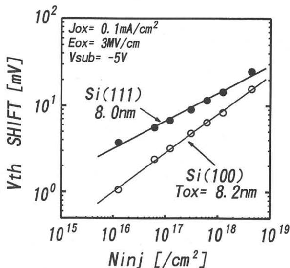
**Figure 3.** The threshold voltage shift of n-MOSFET as a function of the number of injected electrons.
