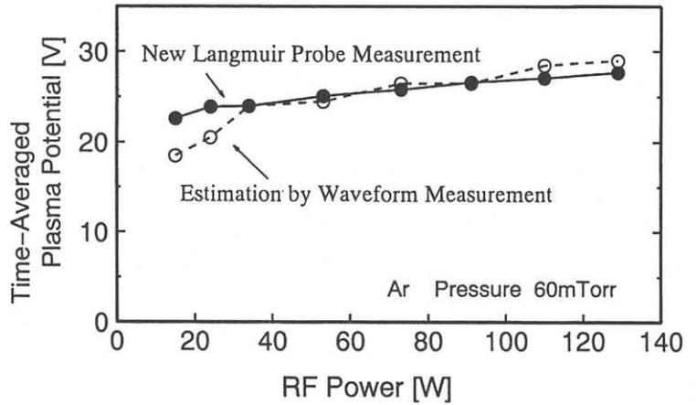
Figure 4 The rf input-power dependence of the time-averaged plasma potential which is measured by newly developed rf Langmuir probe and estimated from voltage waveform of plasma excitation electrode.
