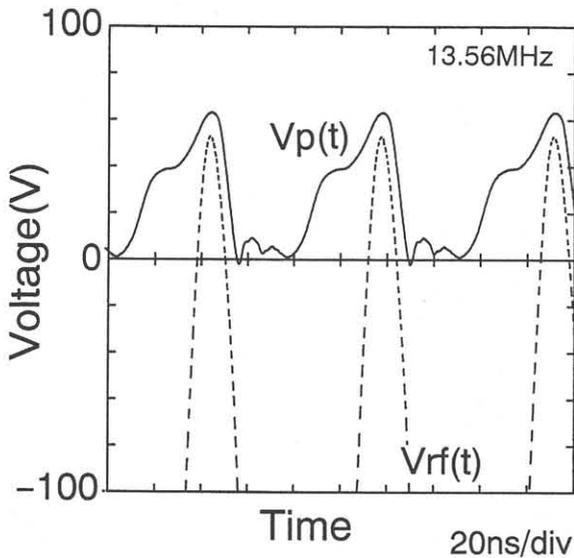
Figure 3 The waveforms of plasma potential  $V_p(t)$  and excitation electrode voltage  $V_{rf}(t)$  at 60mTorr in argon. The rf input-power is 90W.
