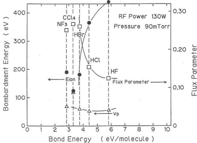
Figure 1 Relationship between bond energy and estimated plasma parameters, such as ion bombardment energy( $E_{ion}$ ), flux parameter and the time-averaged plasma potential( $V_p$ ).
