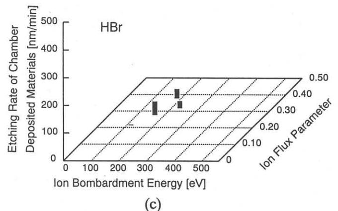
Figure 2 The etching rate of a mixture of photoresist and an OCD silica solution modeled sub-products of etching chamber for  $NF_3$ (a),  $CCl_4$ (b) and  $HBr$ (c).
