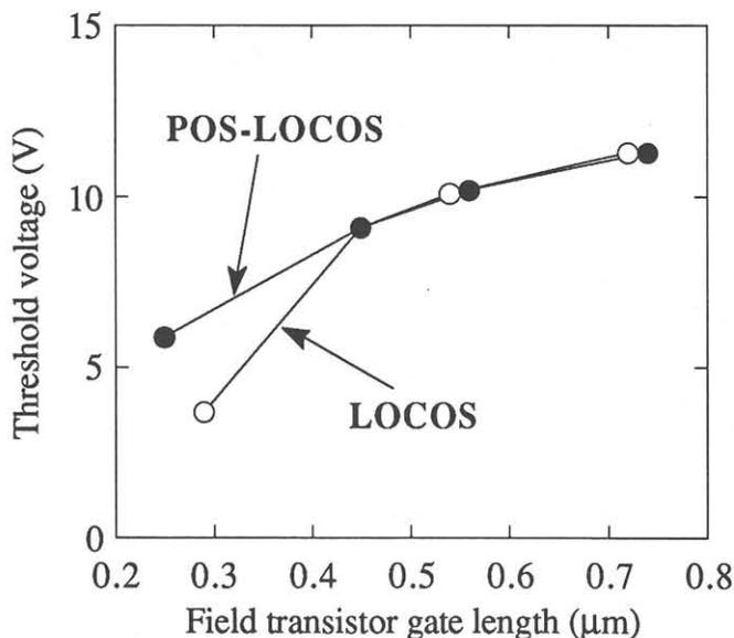
Figure 5. Threshold voltages ( $V_t$ ) of field transistors according to the isolation size.  $W$  is 100  $\mu\text{m}$ ,  $V_d$  and  $V_{\text{sub}}$  are 3.3 V, 0 V, respectively.  $V_t$  was defined as the gate voltage when  $I_d = 1 \mu\text{A}$ .
