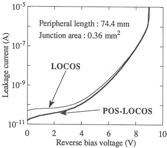
Figure 6. Junction leakage currents of the N<sup>+</sup>/P junctions with LOCOS and POS-LOCOS.
