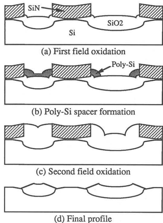
Figure 1. Process steps for POS-LOCOS.
