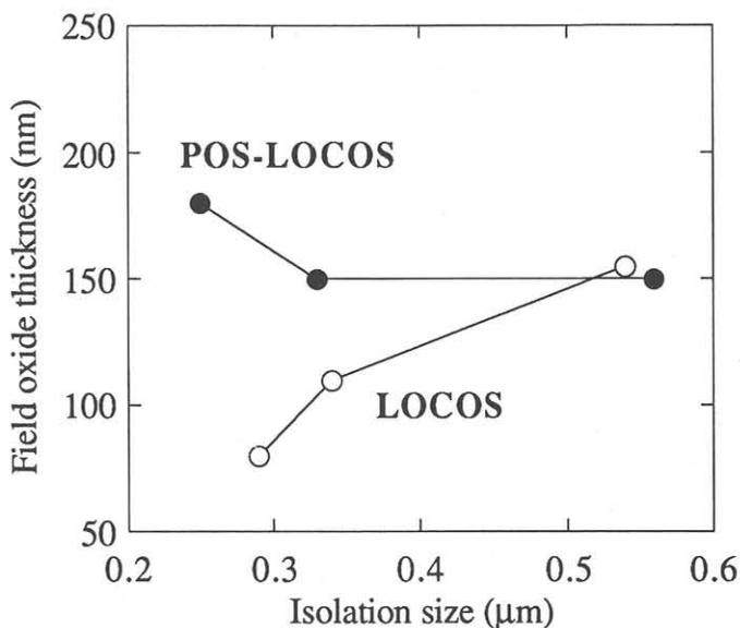
Figure 4. Field oxide thicknesses with respect to the isolation size. The first and the second oxidation thicknesses were both 200 nm at wide isolation regions for POS-LOCOS, and the same oxidation steps were carried out for conventional recessed LOCOS.
