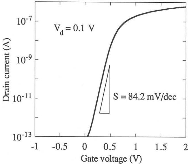
Figure 7.  $I_d$ - $V_g$  characteristic of an NMOSFET with  $L = 10$   $\mu$ m and  $W = 0.3$   $\mu$ m at  $V_d = 0.1$  V, and  $V_{sub} = 0$  V. Gate oxide thickness is 8 nm.
