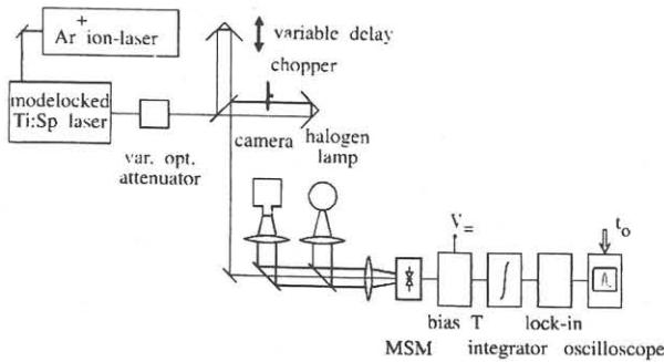
Fig. 1: Optical set-up of the correlation experiments
