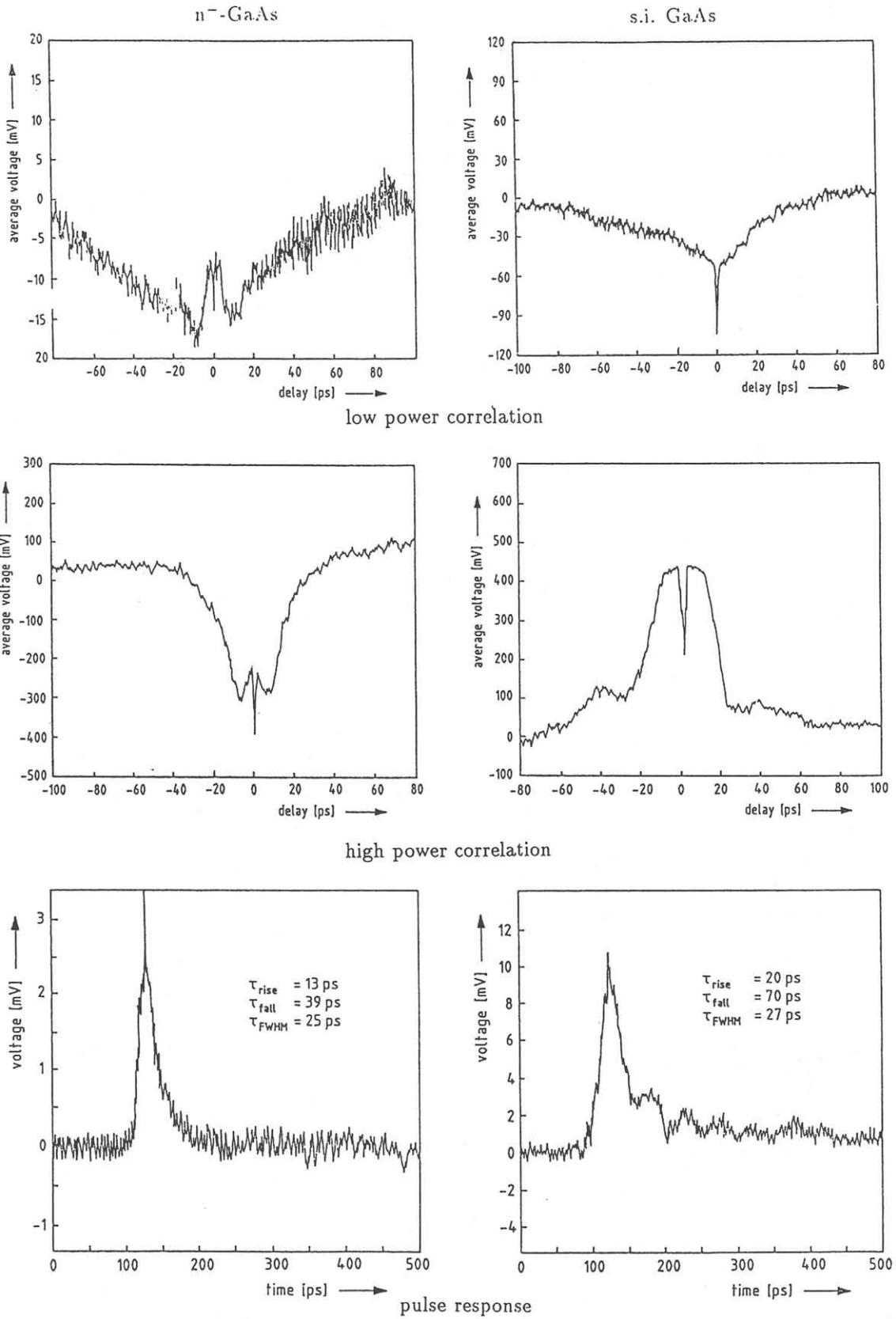
Fig. 2: Correlation functions and pulse response of MSM-photodetectors using undoped and semiinsulating GaAs-materials.
