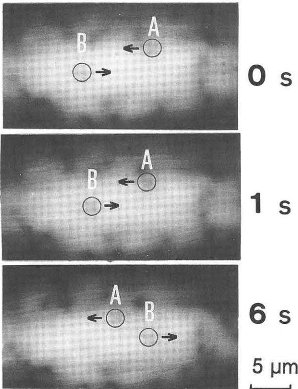
**Fig.2** Dark spots in planar GaAs on Si measured by PLI. The spots marked A and B are moving parallel in the opposite directions.
