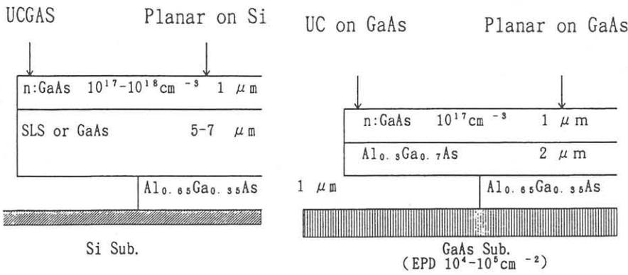
**Fig.1** Sample structure used in the PLI measurement.
