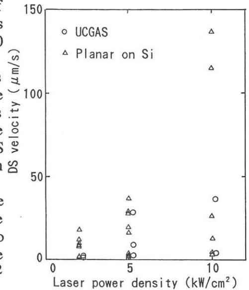
Fig.4 DS velocity as a function of excitation laser power.
