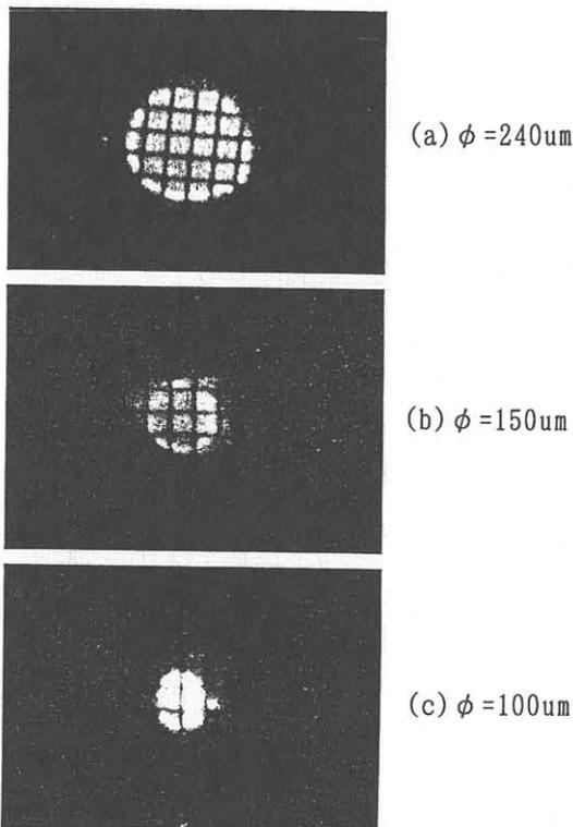
Fig.5 Observed emitted light from bonded LEDs with current of 0.1mA changing the LED size.
