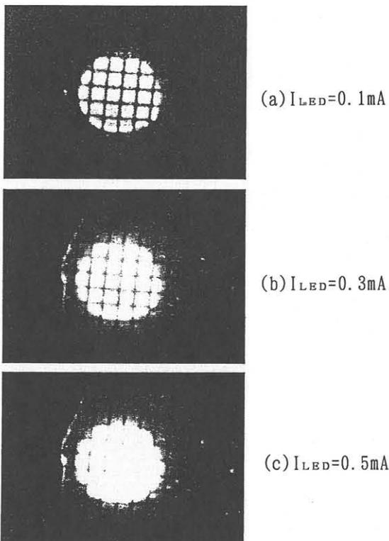
Fig.6 Observed emitted light from bonded LEDs with the diameter of 240µm changing the LED current.
