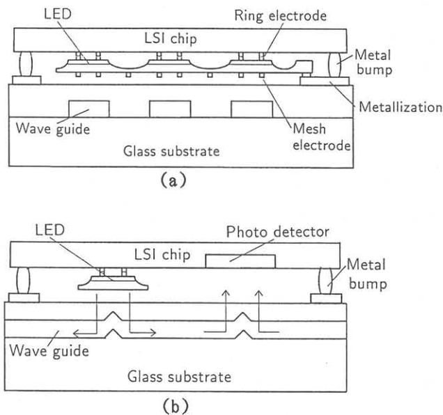
Fig.3 Cross-sectional structure of ORAM-bus memory. (a) Vertical direction to the optical wave guides. (b) Horizontal direction along the optical wave guides.
