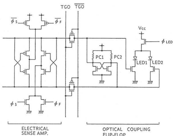
Fig.2 Optical coupling sense amplifier
