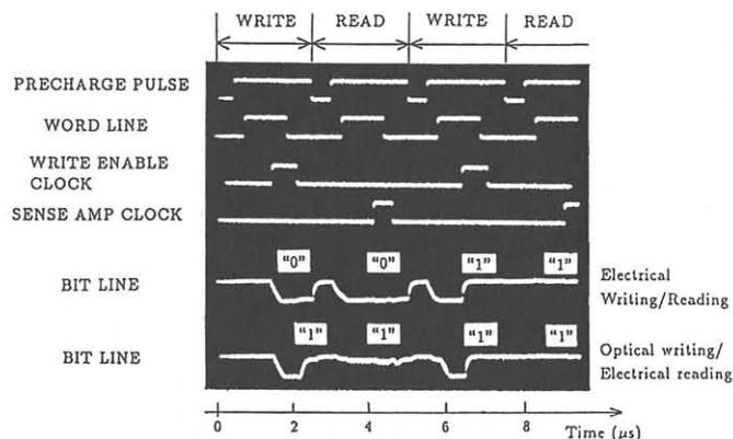
Fig.7 Measured operation waveforms in ORAM-bus memory test chip.
