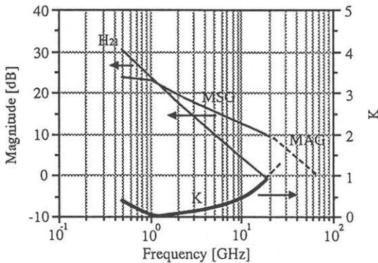
Fig 4. Measured frequency characteristics of GaAs DIBFET with  $L_G = 0.8 \mu m$  and  $W_G = 100 \mu m$  ( $f_T = 16.7 GHz$ ,  $f_{max} = 67GHz$ )
