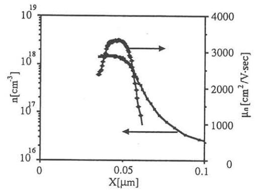
Fig 2. Electron concentration and electron drift mobility profile obtained from C-V and FATFET measurements. The abscissa is the distance from gate.
