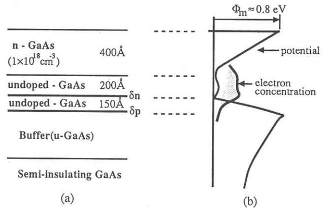
Fig 1. (a) The layer structure of GaAs Dipole-Barrier (DIB)FET and (b) the schematic of electron concentration and potential profile with respect to Fermi-level from one-dimensional analysis. ( $\delta_n=5 \times 10^{12} \text{cm}^{-2}$ ,  $\delta_p=3 \times 10^{12} \text{cm}^{-2}$ )
