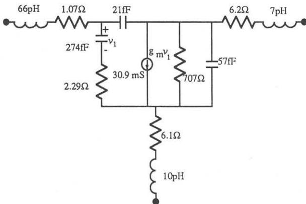
Fig.5 Small-signal equivalent circuit of DIBFET
