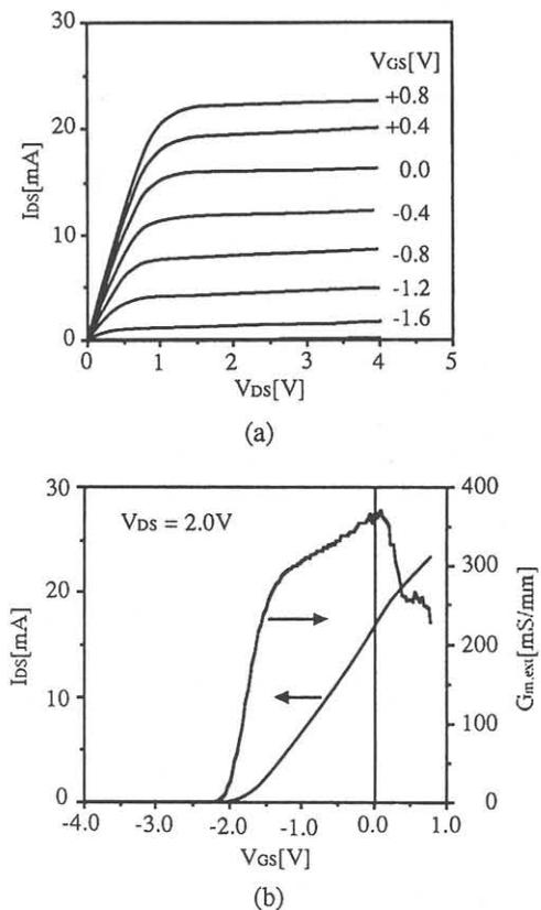
Fig.3 (a) Drain characteristics and(b) transfer characteristics of the fabricated GaAs DIBFET ( $L_G = 0.8 \mu\text{m}$ ,  $W_G = 30 \mu\text{m}$ )
