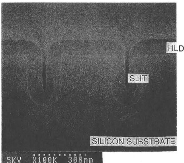
Fig. 2 SEM micrograph of the cross sectional structure after HLD SiO<sub>2</sub> deposition and "slit etch back"
