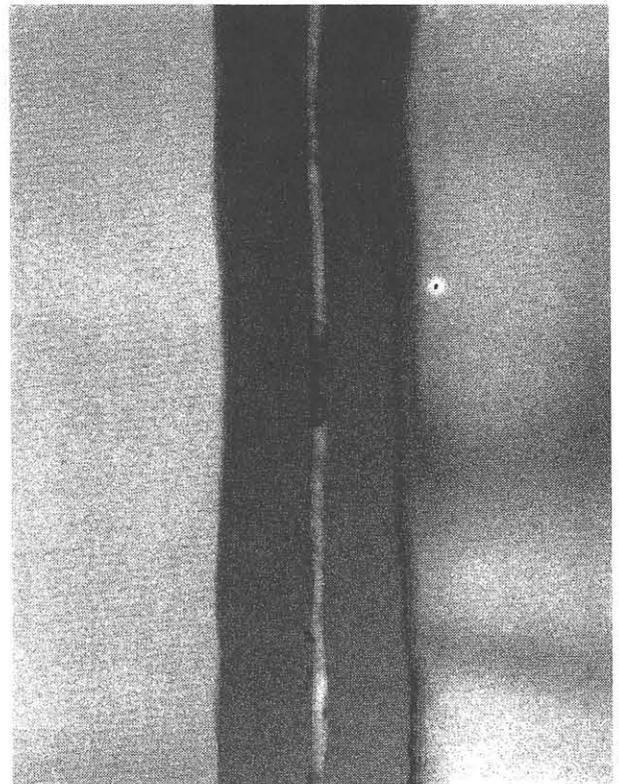
Fig. 5 Plan view TEM micrograph depicting the grain structure of the "slit nano wire" annealed at 1000 C for 10 min.
