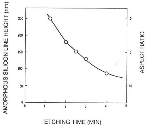
Fig. 3 Etching time dependence of the remaining doped a-Si layer thickness : etching rate decreases with the increase of aspect ratio
