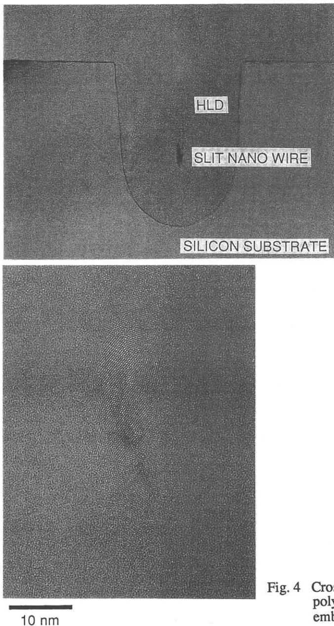
Fig. 4 Cross section TEM micrographs of the polycrystalline silicon "slit nano wire" embedded in the  $\text{SiO}_2$  layer
