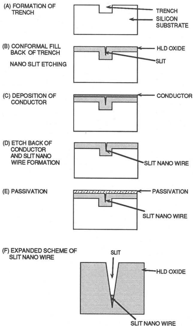
Fig. 1 Schematic presentation of "slit nano wire" fabrication process
