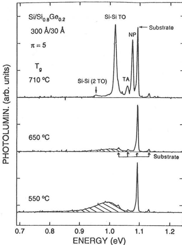
Fig. 1. PL of SiGe heterostructures composed of five 3 nm  $\text{Si}_{0.8}\text{Ge}_{0.2}$  quantum wells separated by 30 nm Si. grown at 550, 650, and 710°C. PL was measured at 1.6 K.
