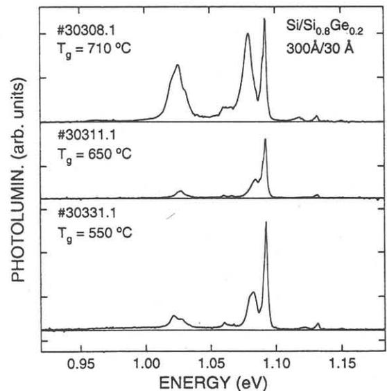
Fig. 3. PL of SiGe heterostructures composed of five 3 nm  $\text{Si}_{0.8}\text{Ge}_{0.2}$  quantum wells separated by 30 nm Si. grown at 550, 650, and 710°C after growth system repairs. PL was measured at 1.6 K.
