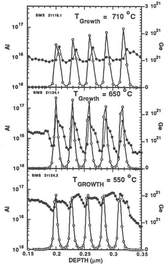
Fig. 2. SIMS profiles of  $\text{Si}_{0.8}\text{Ge}_{0.2}$  quantum wells grown at 550, 650, and 710°C. The solid circles represent Al and the open circles represent Ge.
