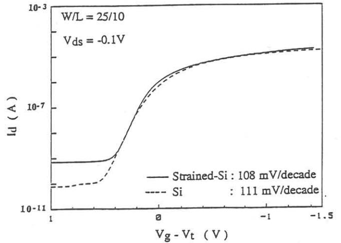
Fig. 6 : Comparison of subthreshold slopes of long-channel Si and strained-Si devices ( $W/L=25/10$ ).
