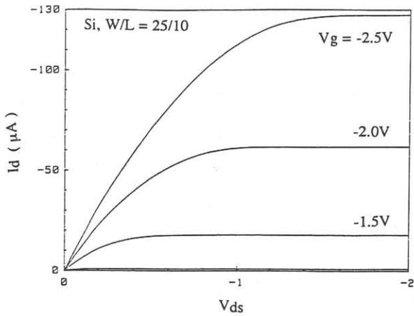
Fig. 3 : I-V characteristics of a long-channel bulk Si device ( $W/L=25/10$ ).
