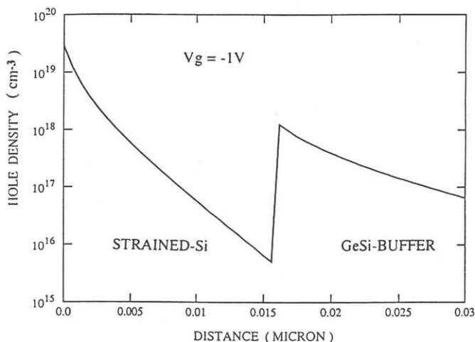
Fig. 2 : 1-D simulation of hole distribution for a gate voltage,  $V_g=-1\text{V}$ .
