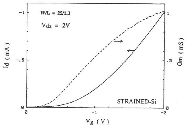
Fig. 8 : Saturation transconductance ( $V_{ds}=-2V$ ) and drain current of a short-channel strained-Si device ( $W/L=25/1.3$ ).
