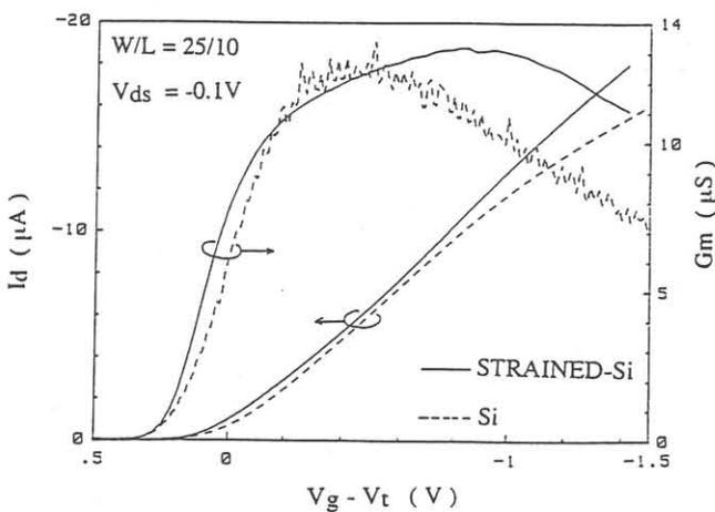
Fig. 5 : Comparison of drain current and linear transconductance for long-channel Si and strained-Si devices ( $W/L=25/10$ ).
