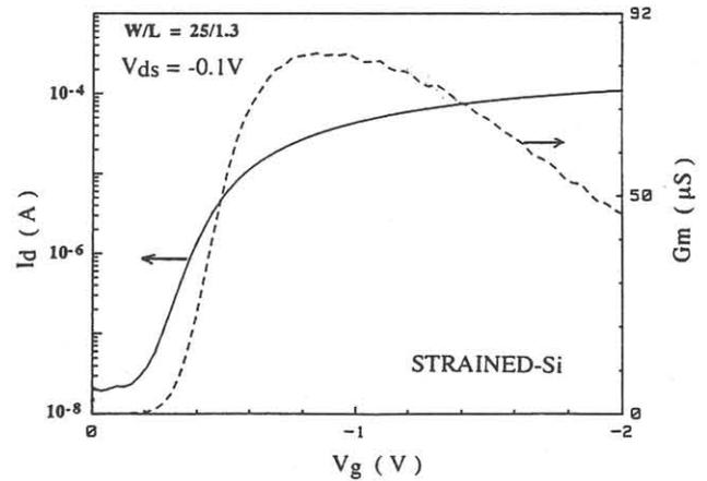
Fig. 7 : Linear transconductance and subthreshold slope of a short-channel strained-Si device ( $W/L=25/1.3$ ).
