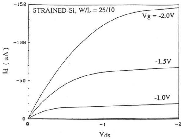
Fig. 4 : I-V characteristics of a long-channel strained-Si device ( $W/L=25/10$ ).
