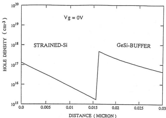
Fig. 1 : 1-D simulation of hole distribution for a gate voltage,  $V_g=0\text{V}$ .
