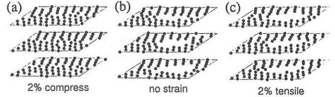
Fig.3 Stability of a void in an equi-directional strain in (001) bicrystal with  $\Sigma=5$ .
