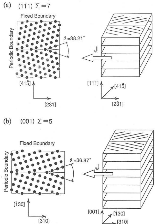
Fig.1 Schematic diagrams of computational cells.
