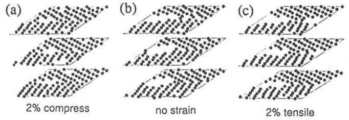
Fig.2 Stability of a void in an equi-directional strain in (111) bicrystal with  $\Sigma=7$ .
