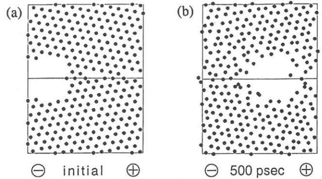
Fig.6 Void movement due to electromigration at the grain boundary.  $1 \times 10^{10} \text{A/cm}^2$ , 700K.
