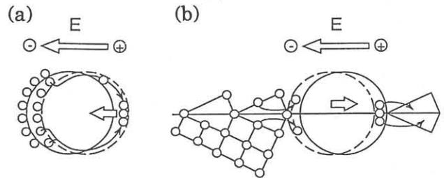
Fig.7 Illustration showing the atomistic view of the direction of the void movement. (a) surface diffusion, (b) grain boundary diffusion.
