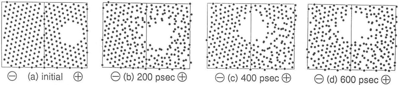
Fig.5 Void movement due to electromigration in the lattice.  $1 \times 10^{10} \text{A/cm}^2$ , 700K.
