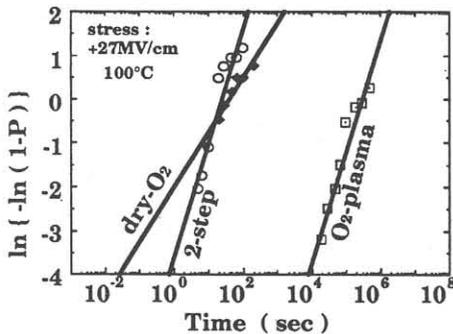
Fig. 7 TDDDB stress time dependence of cumulative failure for O<sub>2</sub>-plasma, dry-O<sub>2</sub> and 2-step
