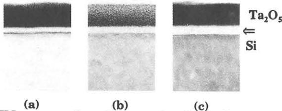
Fig. 5 TEM cross section photographs, (a) as-deposited, (b) O<sub>2</sub>-plasma annealed, and (c) dry-O<sub>2</sub> annealed films (  $\leftarrow$  ; interface layer, 100Å )
