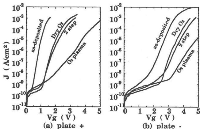
Fig. 1 Leakage current characteristics of the Ta<sub>2</sub>O<sub>5</sub> capacitors.
