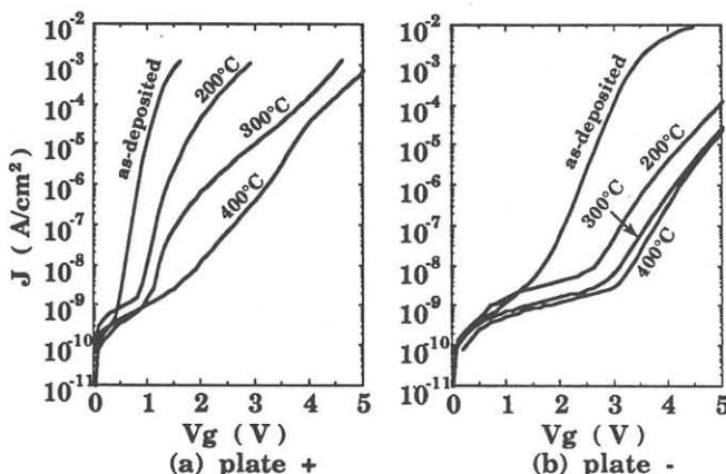
Fig. 2 Annealing temperature dependence of the leakage characteristics for the Ta<sub>2</sub>O<sub>5</sub> capacitor fabricated by O<sub>2</sub> plasma
