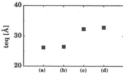
Fig. 6 Changes in  $t_{eq}$  for (a) as-deposited, (b) O<sub>2</sub>-plasma, (c) Dry-O<sub>2</sub>, and (d) 2-step annealed capacitors
