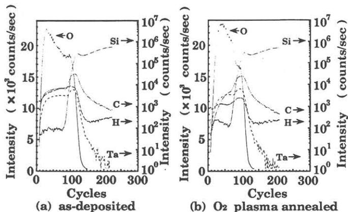
Fig. 3 Depth profiles by SIMS of as-deposited film and O<sub>2</sub> plasma annealed film
