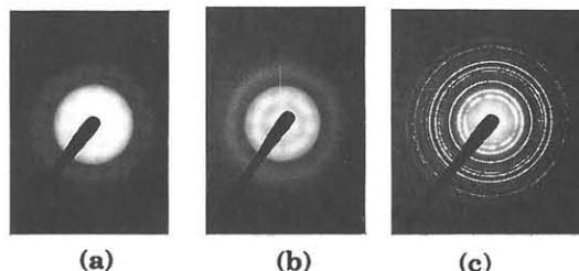
Fig. 4 TED patterns of the Ta<sub>2</sub>O<sub>5</sub> films, (a) as-deposited, (b) O<sub>2</sub>-plasma annealed, and (c) dry-O<sub>2</sub> annealed
