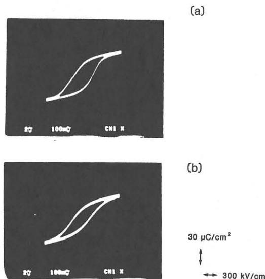
Fig.6. Hysteresis loops of the PZT films 630 Å in thickness on (a) Pt/MgO and (b) Pt/Ti/SiO<sub>2</sub>/Si substrates. Pr and Ec are 23  $\mu\text{C}/\text{cm}^2$ , 240 kV/cm for Pt/MgO, and 18  $\mu\text{C}/\text{cm}^2$ , 200 kV/cm for Pt/Ti/SiO<sub>2</sub>/Si respectively.
