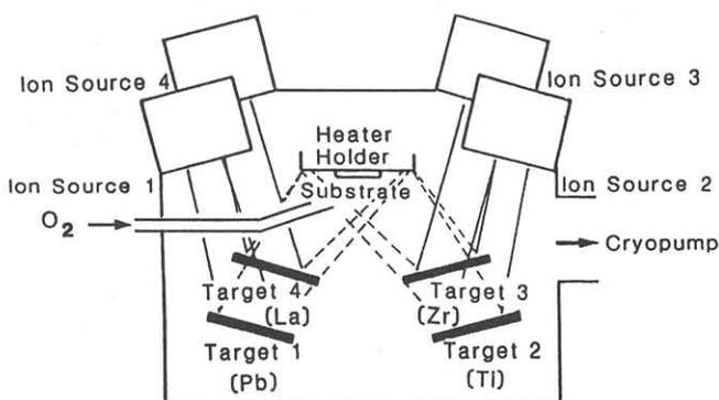
Fig.1. Schematic illustration of multi-ion beam sputtering system.
