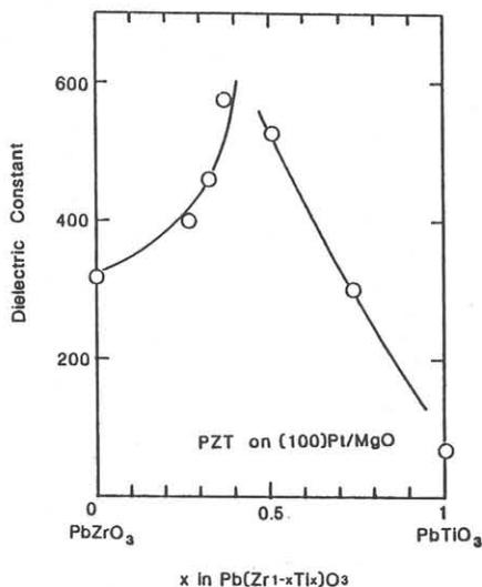
Fig.5. The dielectric constant of c-axis oriented PZT films as a function of Zr/Ti ratio.
