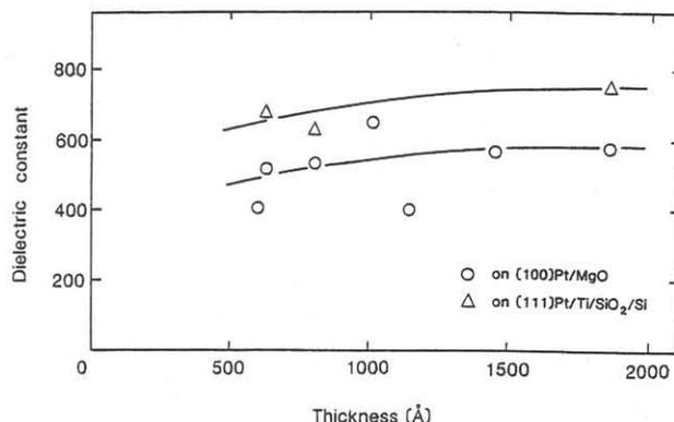
Fig.4. The dielectric constant of the PZT films as a function of the film thickness.
