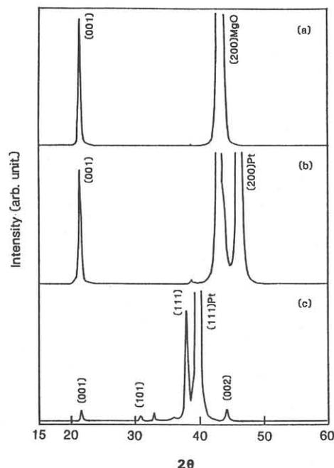
Fig.3. X-ray diffraction patterns of PZT films with PLT buffer layer. The films were deposited on (a) (100)MgO, (b) (100)Pt/MgO and (c) (111)Pt/Ti/SiO<sub>2</sub>/Si substrates.
