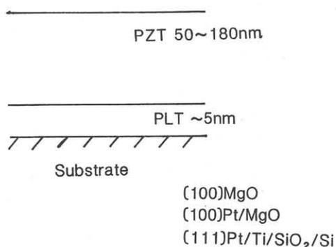
Fig.2. Cross-sectional view of the deposited film.
