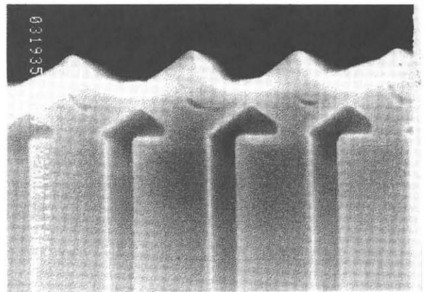
Fig. 3. SEM photograph taken after growing a wire structure sandwiched between AlGaAs layers on the triangular prisms.
