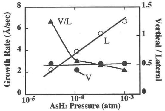
Fig. 2.  $\text{AsH}_3$  pressure dependence of growth rate for vertical (toward (110)) and lateral (perpendicular to (110)) directions. The vertical / lateral ratio is also plotted.
