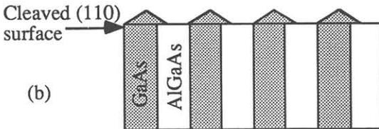
Fig. 1. SEM photograph of selective growth GaAs on the cleaved surface of AlGaAs/GaAs superlattice (a) and its schematic of the structure (b).
