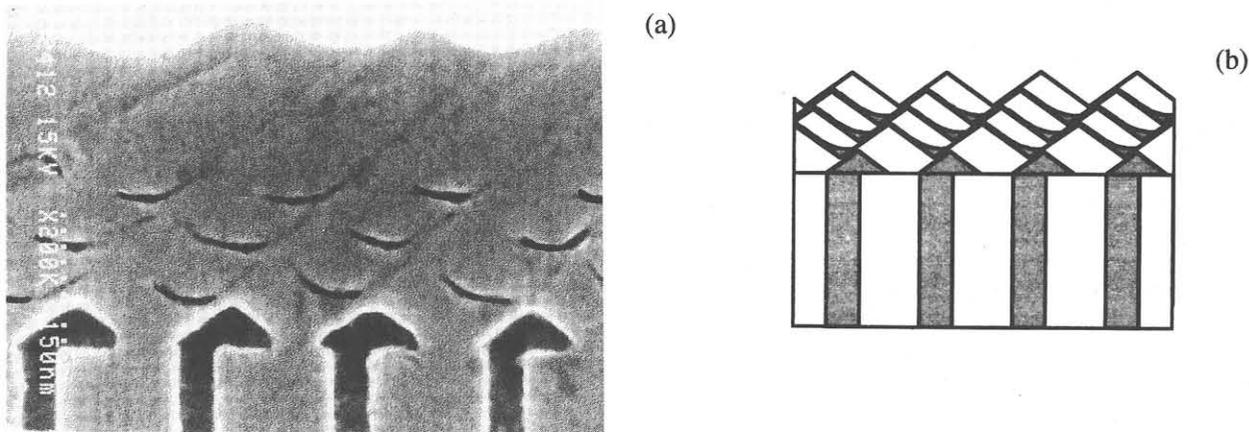
Fig. 4. Fabricated stacked-wire structure on the cleaved facet of AlGaAs/GaAs superlattice (a) and a schematic of the stacked wires (b).
