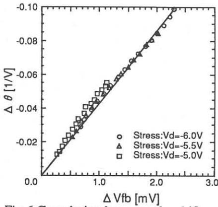
Fig.6 Correlation between the shift on flat-band voltage( $\Delta V_{fb}$ ) and the shift on vertical electric field dependence of effective mobility ( $\Delta\theta$ ).
