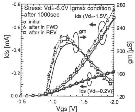
Fig.1 Measured  $I_{ds}$  and  $g_m$  shifts induced by hot carrier compared with the initial in the forward and the reverse operation mode.
