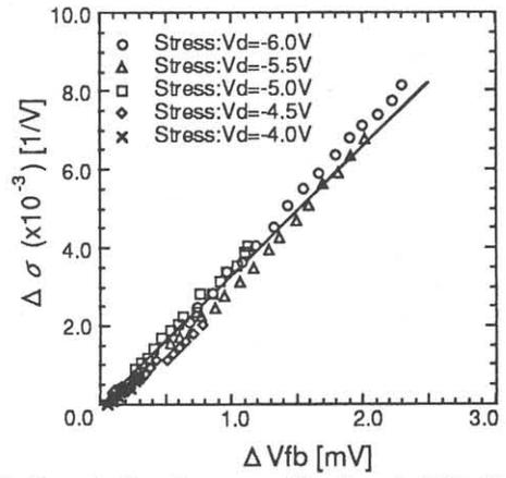
Fig.5 Correlation between flat-band shift ( $\Delta V_{fb}$ ) and TIBL shift ( $\Delta\sigma$ ) in the reverse operation mode at various stress conditions.
