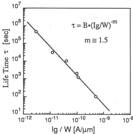
Fig.4 Power law on PMOSFET's hot carrier degradation. Life time  $\tau$  is defined by flat-band shift;  $\Delta V_{fb} = 10\text{mV}$ .
