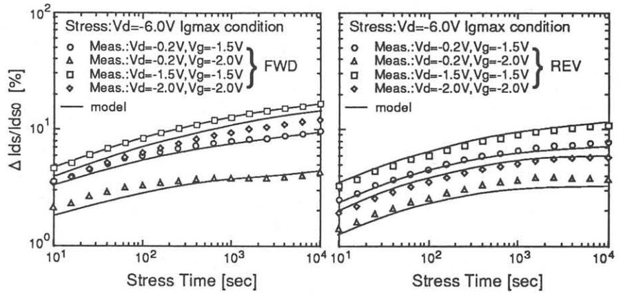
Fig.7 Comparison between measured  $I_d$  shift and calculated  $I_d$  shift by our model. (a) forward operation mode. (b) reverse operation mode.
