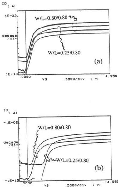
Figure 6 Subthreshold characteristics of narrow devices  $W=0.25\mu\text{m}$  and  $W=0.8\mu\text{m}$  ( $L=0.8\mu\text{m}$ ):
