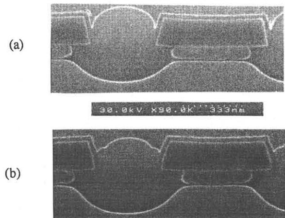
Figure 1 SEM cross section of 1 $\mu$ m pitch array steam oxidized at 1100°C Poly Buffer LOCOS : (a) NOE PBL ; (b) TSE PBL
