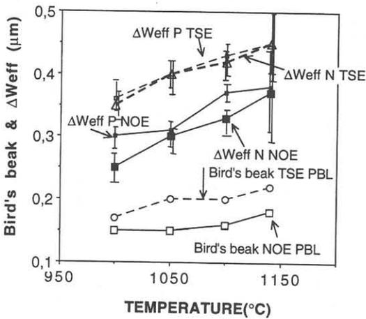
Figure 3 Bird's beak and NMOS, PMOS  $\Delta W_{eff}$  dependance on steam oxidation temperature. NOE PBL and TSE PBL.
