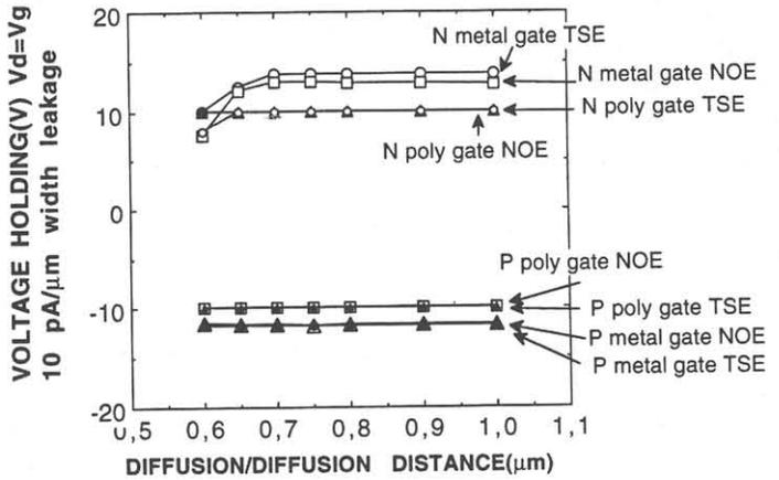
Figure 7 Poly and metal gate field transistors clamping as a function of diffusion separation distance. Field oxidation at  $1100^\circ\text{C}$ .
