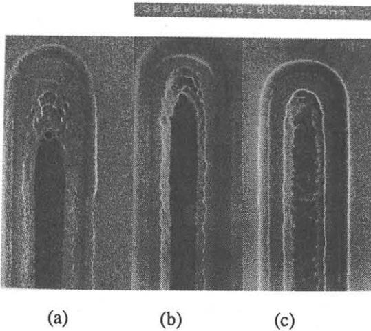
Figure 2 SEM top view of 0.25µm TSE PBL finger pattern for different field oxidation temperatures: (a) 1050°C; (b) 1100°C (c) 1140°C
