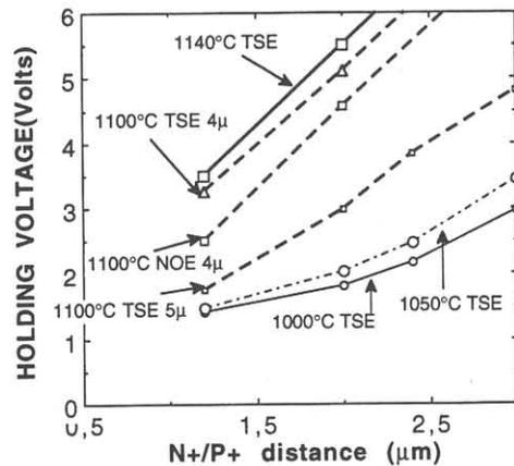
Figure 8 Holding voltage for n+/P-Well/N-Well/P+ structures as a function of n+/p+ distance for different field oxidation temperatures, etch scenario and epi thickness.
