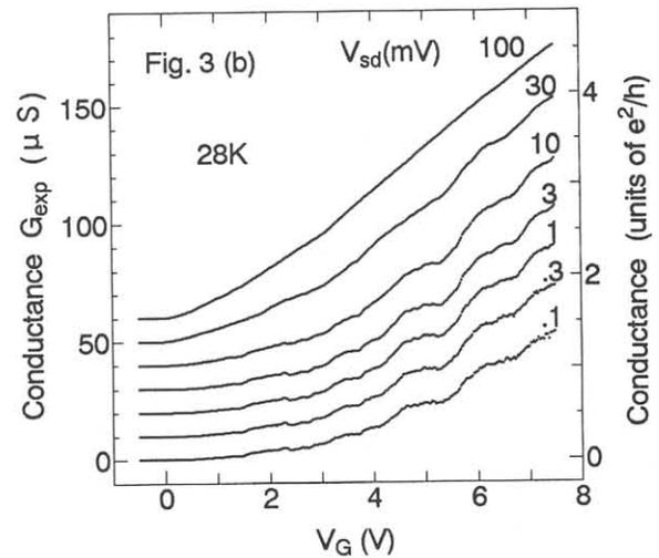
Fig. 3 Gate voltage  $V_g$  dependence of the experimental conductance at various (a) temperatures and (b) source-drain voltages. The curves are offset vertically for clarity.
