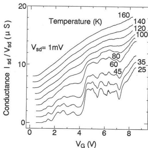
Fig. 5 Gate voltage  $V_g$  dependence of the experimental conductance of the most ultra-fine wire in this work. The curves are offset vertically for clarity.
