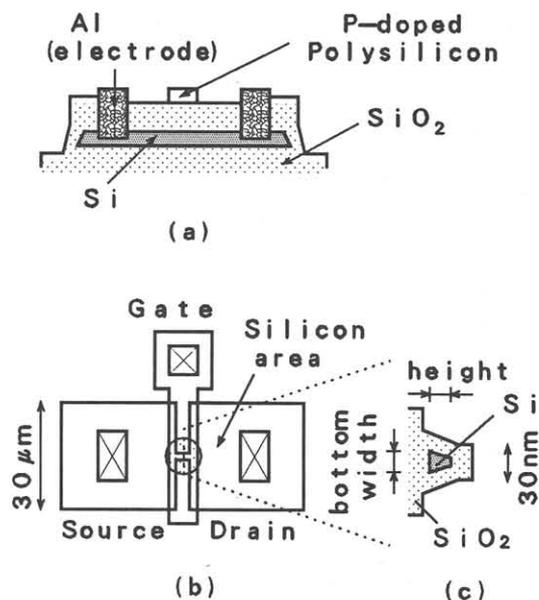
Fig.1 Schematic diagram of the device structure; (a) cross section, (b) top view, (c) expanded cross section of the silicon wire. A silicon quantum wire with a trapezoidal cross-section is formed in the center of the source and drain regions under the gate, shown by the circle in (b).
