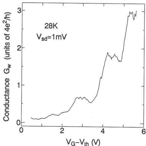
Fig. 4 The wire conductance  $G_w$  as a function of gate voltage  $V_g$ . Series resistance  $G_s^{-1}$  was subtracted.
