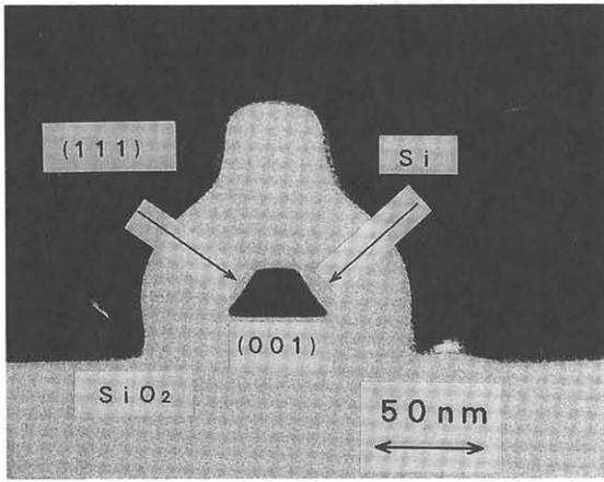
Fig. 2 Cross sectional TEM photograph of the wire.
