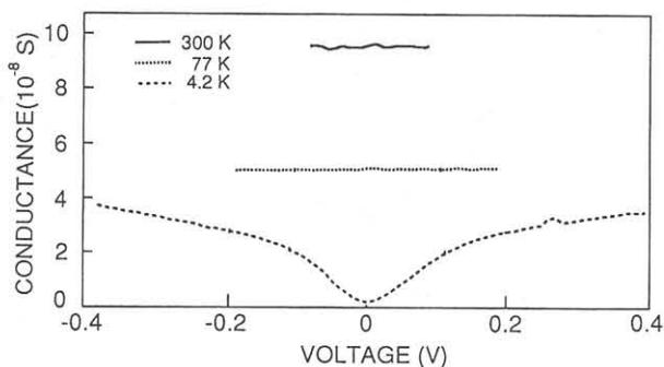
Fig. 5 Conductance of the nano wire at 300 K, 77 K and 4.2 K
