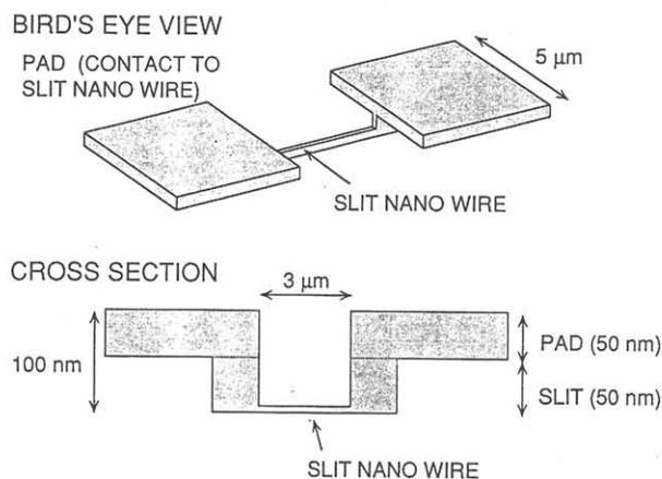
Fig. 3 Schematic drawing of the nano wire device structure
