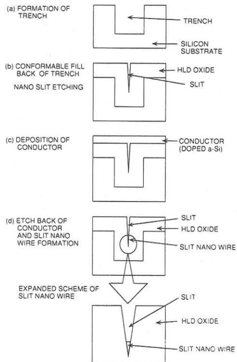
Fig. 1 Cross section of poly-Si nano wire fabrication process
