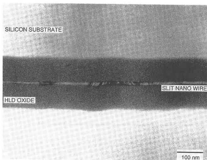
Fig. 2 Plan view TEM micrograph of the nano wire annealed at 1000°C
