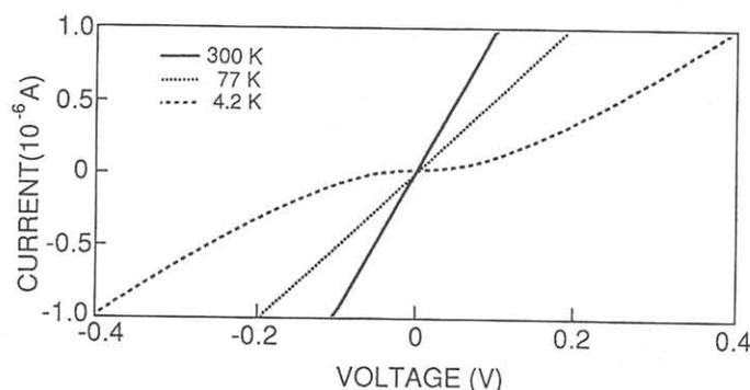
Fig. 4 Current-voltage characteristics of the nano wire at 300 K, 77 K and 4.2 K ; a 30 mV gap appears at 4.2 K
