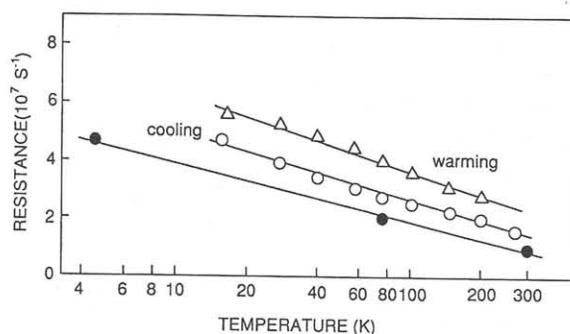
Fig. 6 Conductance analysis based on the weak localization model
