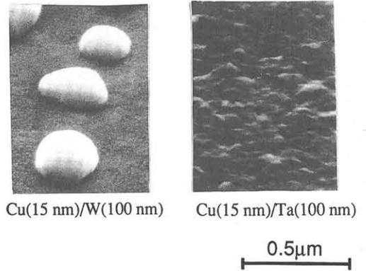
Fig.5 SEM photographs of Cu surface morphology on W and Ta underlayers.
