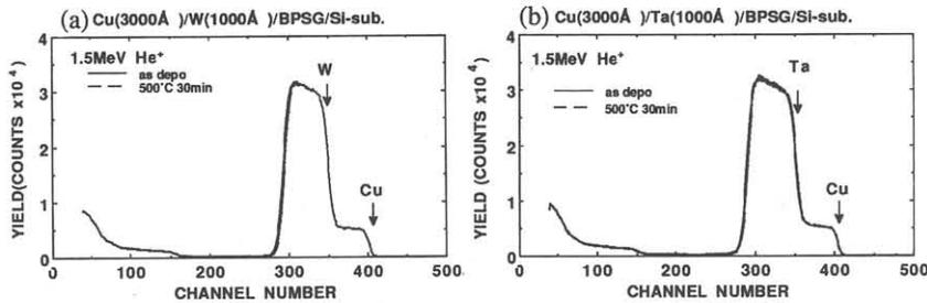
Fig.3 RBS spectra for (a) Cu(300 nm)/W structure and (b) Cu(300 nm)/Ta structure before and after annealing at 500 °C for 30 min.
