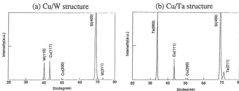
Fig.4 XRD patterns from (a) Cu/W structure and (b) Cu/Ta structure after annealing at 450 °C for 30 min.
