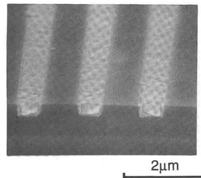
Fig.7 Cross-sectional SEM photograph of Cu/W layered structure after CMP process.
