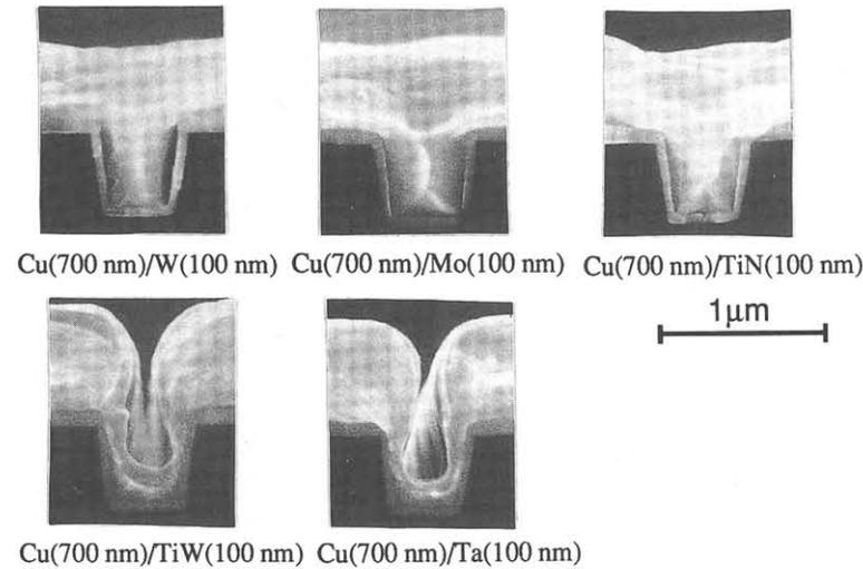
Fig.2 Cross-sectional SEM photographs of Cu stacked structures after annealing at 450 °C for 30 min.
