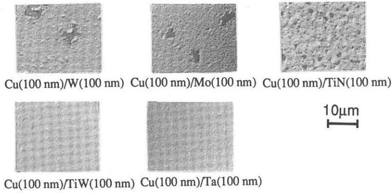
Fig.1 Optical photographs of Cu film (100 nm) on various metal films after annealing at 450 °C for 30 min.
