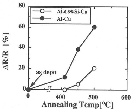
Fig. 2 Sheet resistance changes of Al-0.8%Si-Cu/Ti and Al-Cu/Ti structures as a function of annealing temperature.
