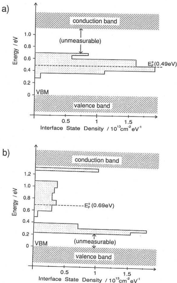
Fig. 3 The energy distribution of the interface states in the band-gap: a) for the (30 Å-Pt/25 Å-silicon oxide/n-Si(100)) device; b) for the (30 Å-Pt/25 Å-oxide/p-InP(100)) device.
