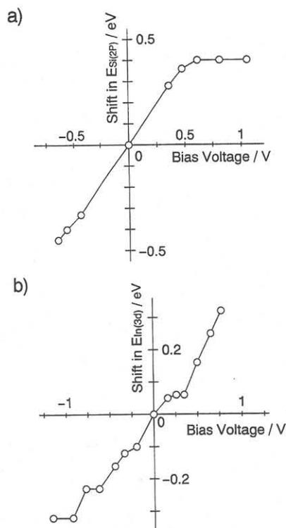
Fig. 2 Amounts of the shift of the Si( $2p_{3/2}$ ) peak (Fig. 2a) and the In( $3d_{5/2}$ ) peak (Fig. 2b) as a function of the bias-voltage.
