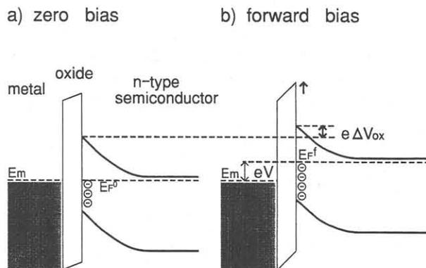
Fig. 1 Band diagrams for an n-type semiconductor-based MOS device: a) at zero bias; b) under a forward bias.
