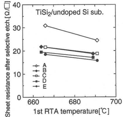
Fig.1: Sheet resistance dependence on the 1st RTA temperature after selective TiN etching.
