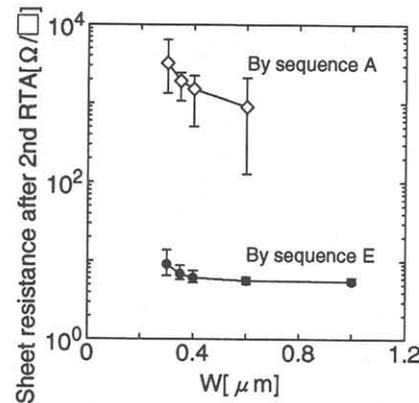
Fig.6: Sheet resistance dependence on the line width for  $\text{TiSi}_2$  films, formed on the  $n^+$  doped poly-Si, with amorphization by As ion-implantation.
