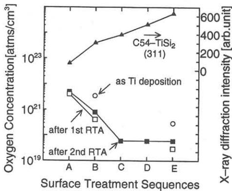
Fig.4: Surface treatment sequence dependence of oxygen concentration by SIMS depth profiles at the  $\text{TiSi}_2/\text{Si}$  interfaces, and of X-ray diffraction intensity for C54- $\text{TiSi}_2$  films, after 2nd RTA at  $810^\circ\text{C}$  with 1st RTA at  $665^\circ\text{C}$ .
