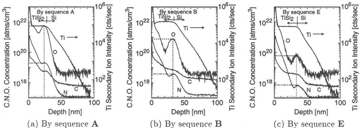
Fig.3: SIMS depth profiles for titanium, oxygen, nitrogen and carbon in  $\text{TiSi}_2$  films, after 2nd RTA at  $810^\circ\text{C}$  with 1st RTA at  $665^\circ\text{C}$ .
