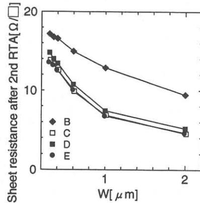
Fig.5: Sheet resistance dependence on the line width for  $\text{TiSi}_2$  films on undoped poly-Si.
