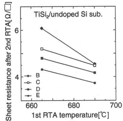
Fig.2: Sheet resistance dependence on the 1st RTA temperature after the 2nd RTA.
