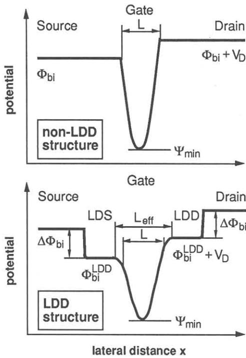
Fig. 4 Schematic illustration of the lateral potential profile for non-LDD and LDD structure showing the built-in potential shift  $\Delta\Phi_{bi}$  and the change in  $L_{eff}$
