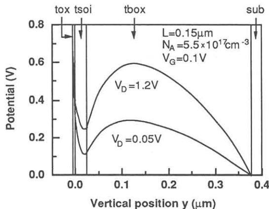
Fig. 2 Simulated vertical potential through the SOI-structure at  $x=L/2$  showing the nonlinearity inside the buried oxide
