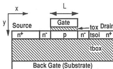
Fig. 1 Schematic cross section of the n-channel SOI MOSFET structure (L=0.15 $\mu$ m, tox=60 $\text{\AA}$ , tsoi=250 $\text{\AA}$ , tbox=3800 $\text{\AA}$ )
