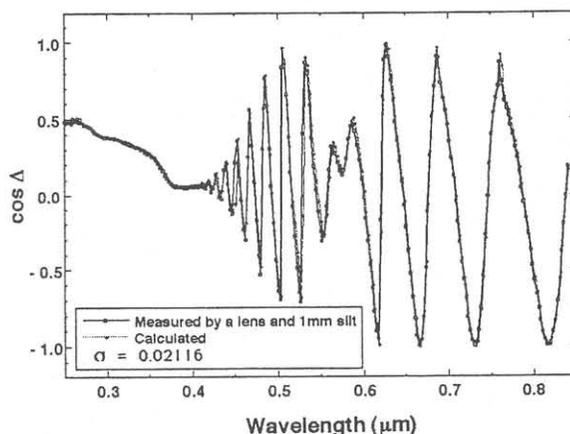
Fig. 2 Best fitting between calculated and measured spectroscopic ellipsometry data for an investigated ONO film on SOI substrate.
