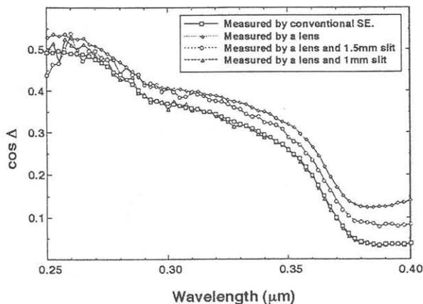
Fig. 1 Spectroscopic ellipsometry data for four kinds of measurement. (i) using a lens of magnification 30x. (ii) using a lens of magnification 30x attached to about 1.5 mm slit width. (iii) using a lens of magnification 30x attached to about 1 mm slit width. (iv) using a conventional setup with a normal spot size of 3 mm.
