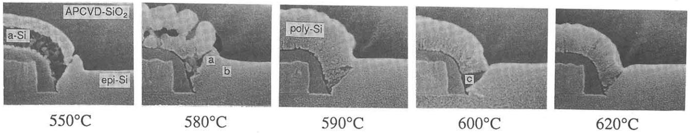
Fig.6 Cross-sectional SEM micrographs of Si layer deposited at various temperatures
