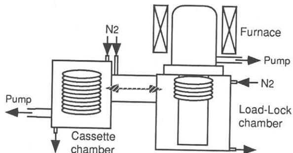
Fig.2 Schematic diagram of the novel "contamination-restrained Load-Lock LPCVD" system
