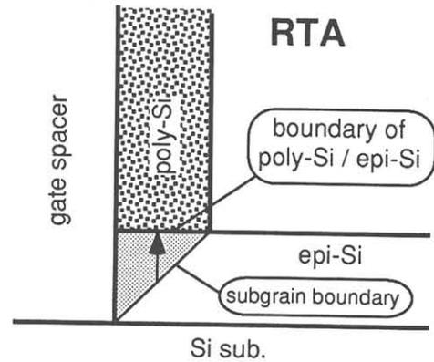
Fig.9 Model of the formation mechanism for the facet-free full-flat elevated S/D
