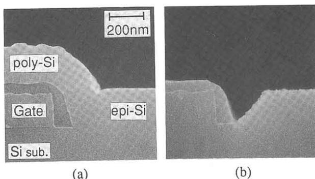
Fig.5 Cross-sectional SEM micrographs of Si layer deposited at 620°C (a) before and (b) after selective etching
