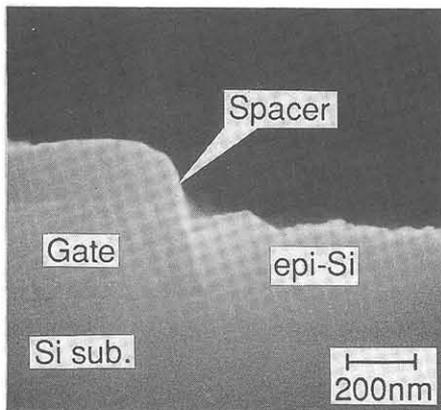
Fig.8 Cross-sectional SEM micrograph of Si layer after selective etching
