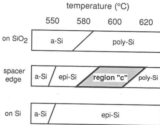
Fig.7 States of Si films deposited at various temperature on each position
