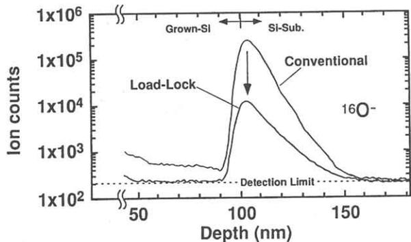
Fig.3 SIMS depth profiles of oxygen ion for the Si films on the Si substrate deposited by conventional LPCVD and L/L LPCVD systems
