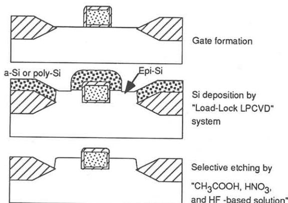
Fig.1 Fabrication procedure of elevated source/drain structure
