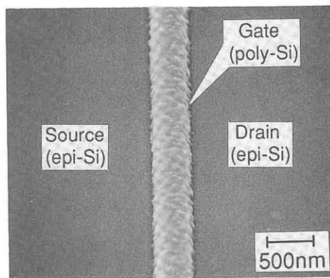
Fig.4 Oblique-directional SEM micrograph of Si layer deposited at 620°C using L/L LPCVD system
