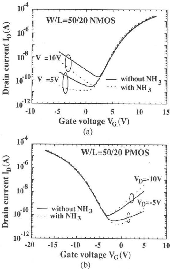
Fig. 2 The  $I_D$ - $V_G$  characteristics of TFT's with  $\text{NH}_3$  annealing at  $800^\circ\text{C}$  for 30 min and without  $\text{NH}_3$  annealing, respectively.
