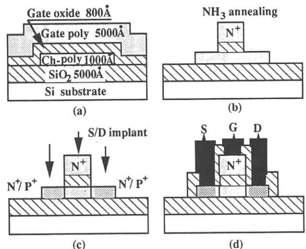
Fig. 1 The main fabrication steps of  $\text{NH}_3$  annealed devices. a) gate poly doping using solid diffusion source (970 °C, 30 min) b)  $\text{NH}_3$  annealing in conventional furnace c)  $\text{N}^+$ ,  $\text{P}^+$  S/D implant d) final device structure (NMOS, PMOS)
