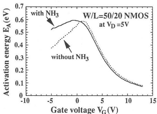
Fig. 4 Activation energy variations with gate voltage for the devices with  $NH_3$  annealing at  $800^\circ C$  for 30 min and without  $NH_3$  annealing. Devices are measured at  $V_D=5V$  in the temperature range of  $20^\circ C$  to  $100^\circ C$ .
