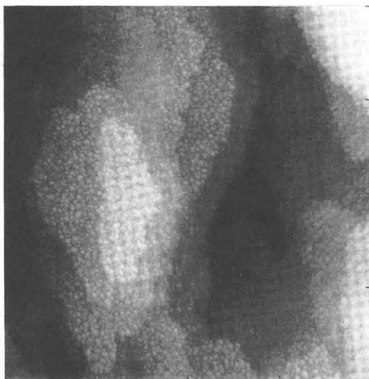
Fig. 1 100x100nm<sup>2</sup> STM image of 0.8ML Fe grown on the c(4x4) reconstructed GaAs(100) surface taken in a constant current mode with a 100pA tunneling current.
