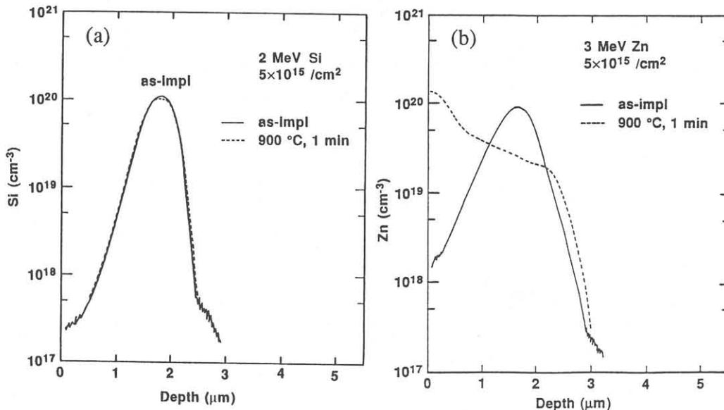
Fig. 4 Depth profiles of Si (a) and Zn (b) before and after annealing at 900 °C for 1 min. Implantation conditions are indicated in the figure.
