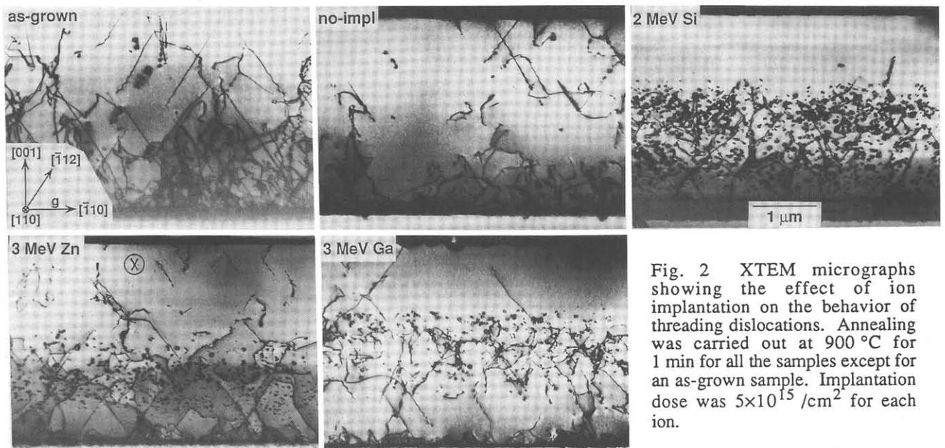
Fig. 2 XTEM micrographs showing the effect of ion implantation on the behavior of threading dislocations. Annealing was carried out at 900 °C for 1 min for all the samples except for an as-grown sample. Implantation dose was  $5 \times 10^{15}$  /cm<sup>2</sup> for each ion.
