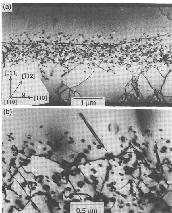
Fig. 5 XTEM micrographs showing the interaction between dislocations and implanted layers for Si implantation results. (a) A sample was annealed at 800 °C for 30 min after implantation at 1.7 MeV with a  $5 \times 10^{15} / \text{cm}^2$  dose. (b) A sample was annealed at 1000 °C for 1 min after implantation at 2 MeV with a  $5 \times 10^{15} / \text{cm}^2$  dose.
