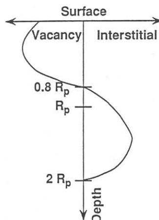
Fig. 1 Schematic drawing of distribution of point defects in the substrate introduced by ion implantation.
