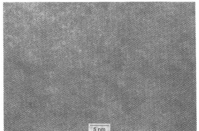
Fig. 3 High-resolution XTEM micrograph showing no defect creation in the as-implanted region, denoted by X in Zn implantation in Fig. 2. [110] projection.
