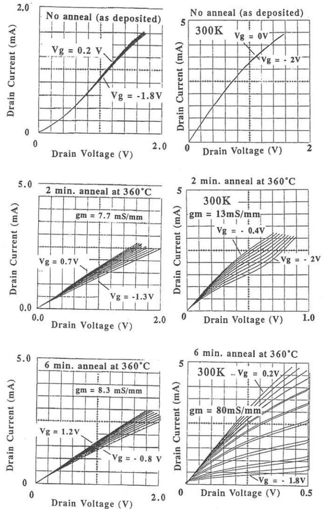
Fig.3. Current voltage characteristics of an InAs heterojunction FET fabricated by "Process A".
