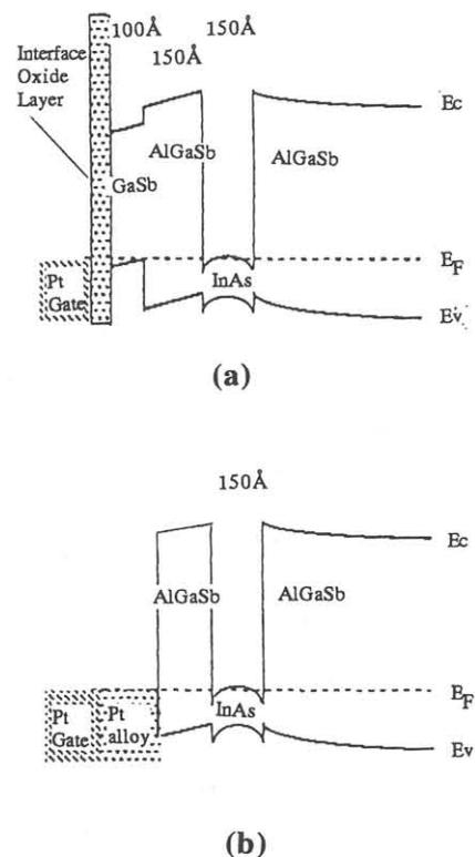
Fig. 5. Schematic energyband diagram of a platinum gated InAs/AlGaSb HFET (a) before and (b) after Schottky gate alloy.
