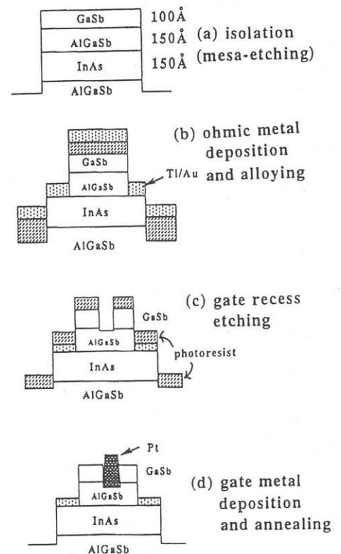
Fig.1. Process flow of InAs heterojunction FET with platinum gate ("Process A")
