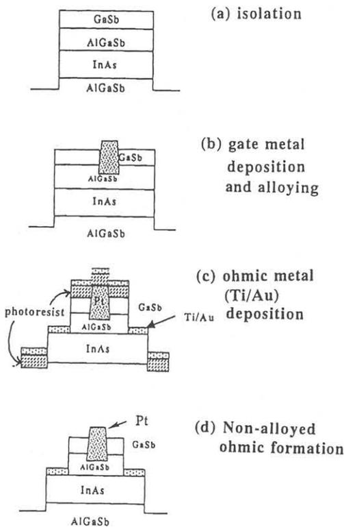
Fig. 2. Process flow of InAs heterojunction FET with platinum gate ("Process B")
