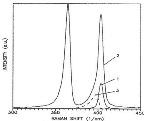
Fig.1 The Raman spectra of initial GaP wafer (1), and porous GaP layer (2). Dashed line (3) shows the result of computer decomposition of LO-phonon line.
