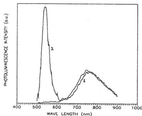
Fig.2 Photoluminescence spectra of initial GaP wafer (1) and porous GaP layer (2).
