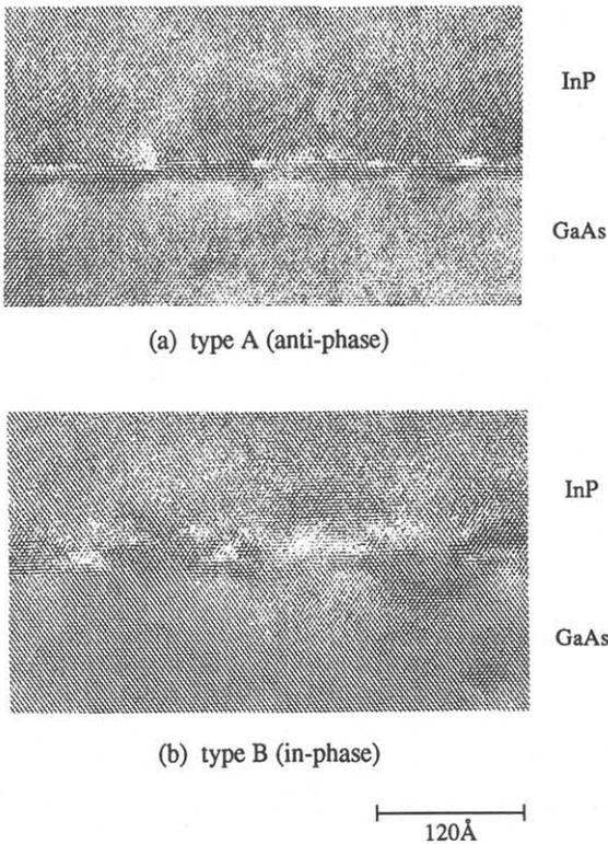
Figure 2 High-resolution cross-sectional TEM images around the InP/GaAs interface: (a) type A, (b) type B.
