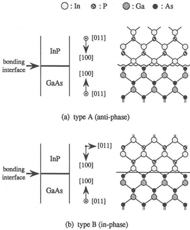
Figure 1 Relation of crystal axes between GaAs and InP wafers with schematic lattice structure: (a) type A, (b) type B. The wavy line in (a) shows the anti-phased boundary, whereas the straight line in (b) shows the in-phase boundary.
