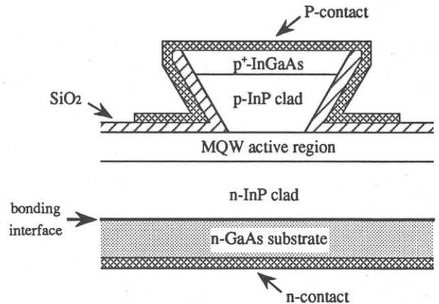
Figure 3 Schematic diagram of 1.55-μm MQW ridge waveguide lasers on GaAs.
