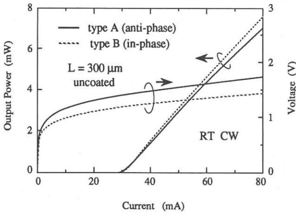
Figure 4 Light-current and voltage-current characteristics of the two types of lasers on GaAs.
