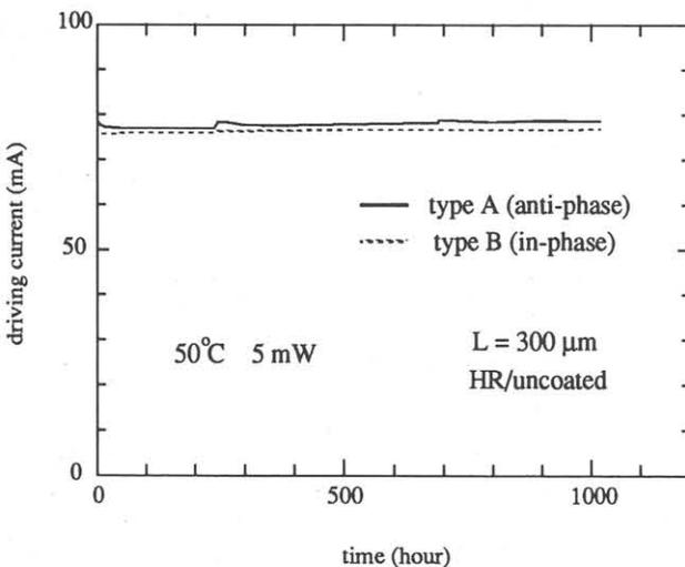
Figure 6 Results of preliminary APC test for the two types of 1.55-μm lasers on GaAs at 50°C.
