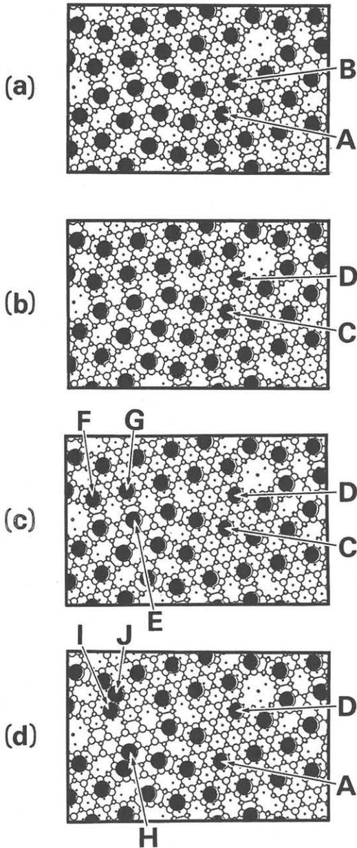
Fig.4 Positions of surface Si atoms observed in Fig.3 (a)-(d). A-J indicate the positions of moved Si atoms before and after the movement [3].
