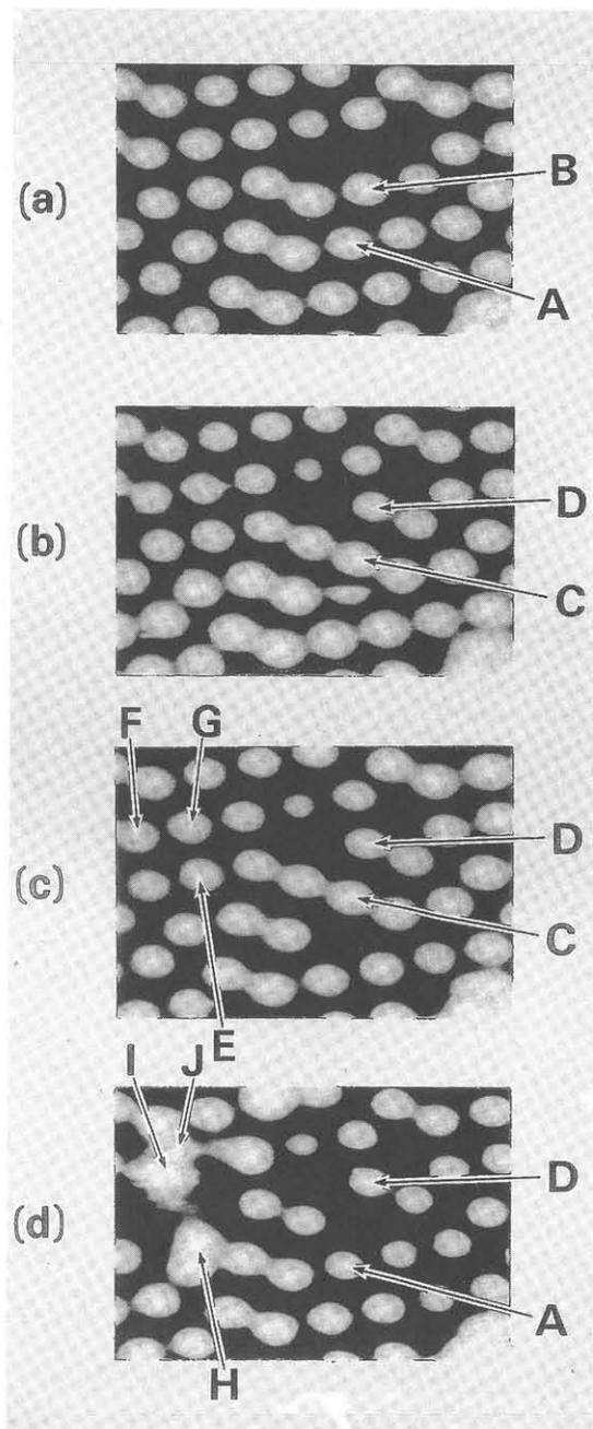
Fig.3 A series of STM images of the Si(111)7x7 surface in a region containing an out-of-phase boundary. Movement of surface Si atoms is observed [3].
