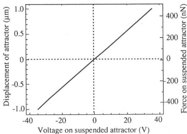
(b). Relationship between voltage, force and displacement for  $85 \mu\text{m}$  long attractors.
