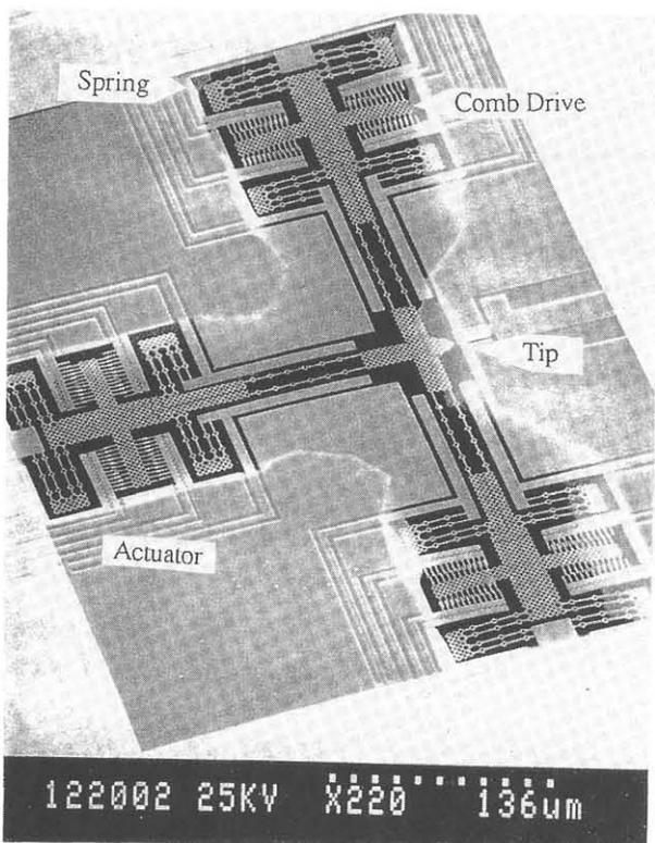
Fig. 4. SEM of 2 dimensional STM chip.
