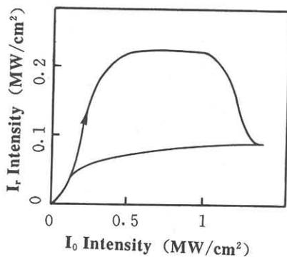
Fig. 3 The optical bistability of ZnS - ZnTe/GaAs MQWs on reflection at room temperature.
