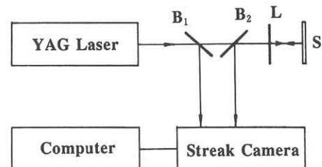
Fig. 1 Schematic diagram for measuring optical bistability in ZnS - ZnTe MQWs on reflection at room temperature; (B) beam splitter; (L) lens; (S) sample.
