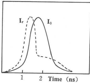
Fig. 2 Time dependence of the normalized temporal shapes of incident (solid curve)  $I_0$  and reflection (dashed curve)  $I_r$  pulses in ZnS - ZnTe/GaAs MQWs at room temperature.
