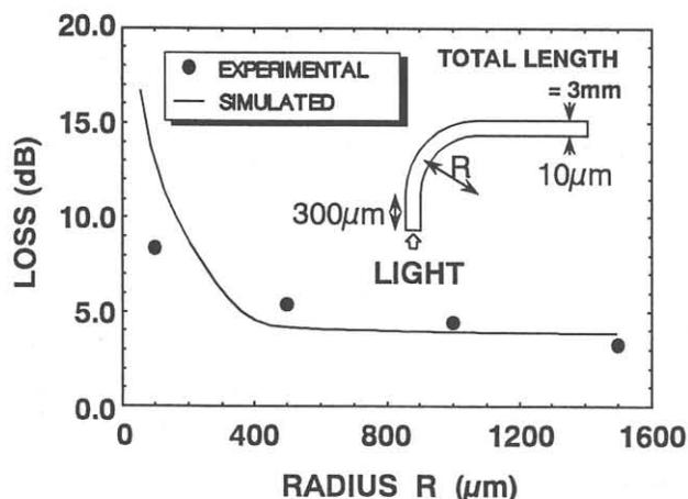
Fig. 7 Bending loss at the corner vs curvature radius.
