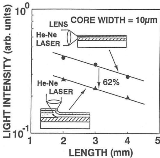
Fig. 3 Output light intensity versus waveguide length for poly-Si mirror and straight waveguide.
