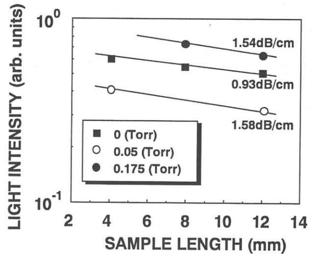
Fig. 5 Light propagation loss for slab waveguides with SiO<sub>x</sub>N<sub>y</sub> core.
