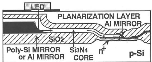
Fig. 1 Detailed structure of OEIC on Si.
