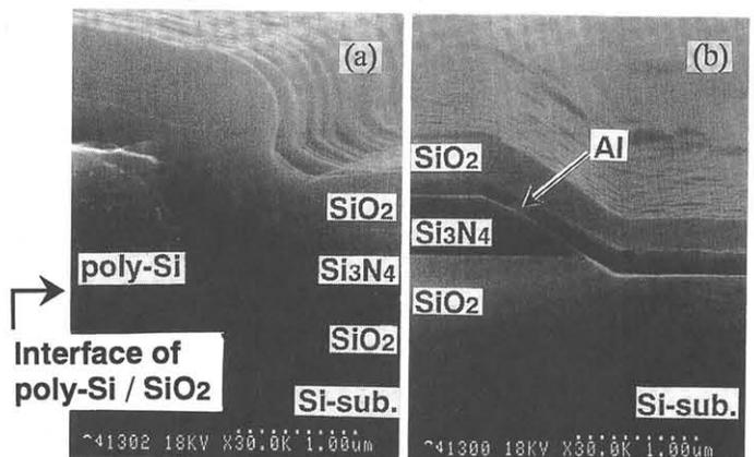
Fig. 2 Cross-sectional SEM photograph of (a) poly-Si mirror and (b) Al mirror.
