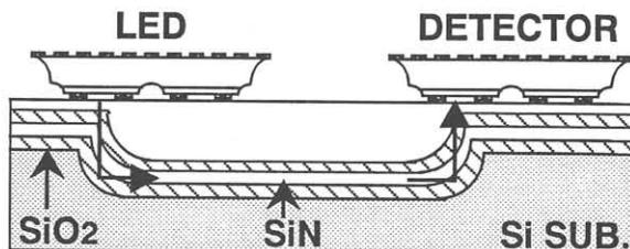
(b) Cross sectional view of fabricated OEIC on Si chip.
