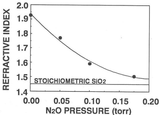
Fig. 4 Refractive index of SiO<sub>x</sub>N<sub>y</sub> vs N<sub>2</sub>O pressure.
