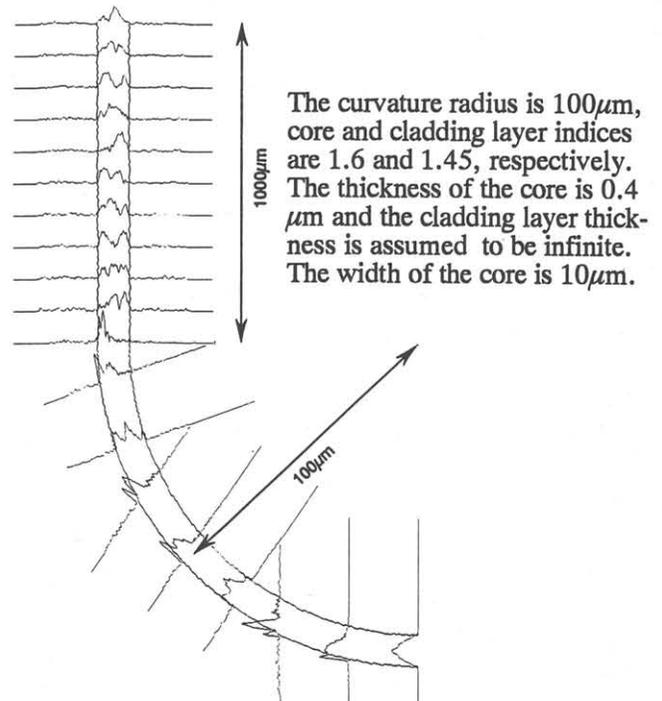
Fig. 6 Simulated result of light intensity profile along a curved waveguide.
