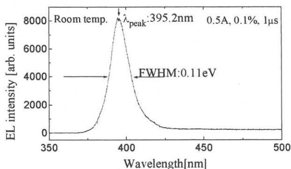
Fig.3 EL spectrum of the devices under high current injection of 0.5A.
