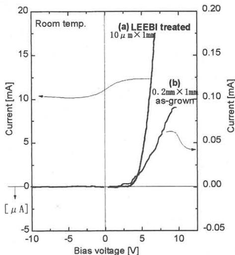
Fig.2 I-V curves of the AlGaIn/GaN/GaInN stacked heterostructure (a) with and (b) without the partial LEEBI treatment. Stripe width of electrode on p-layer is  $200 \mu\text{m}$ . Stripe width of the LEEBI treated region is  $10 \mu\text{m}$ .
