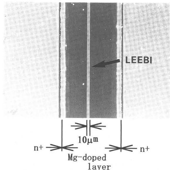
Fig.1 Photograph of fluorescence microscope of sample surface with the partial LEEBI treatment.
