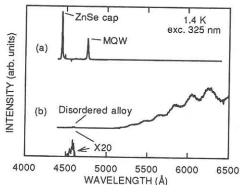
Fig.3 PL spectra (a) for the as-grown  $\text{Cd}_x\text{Zn}_{1-x}\text{Se}/\text{ZnSe}$  SLS; and (b) for the Ne-implanted (400  $^\circ\text{C}$ ) SLS after the ZnSe cap layer was removed by etching in HCl.
