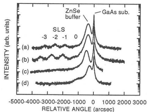
Fig.2 X-ray diffraction profile (a) for the as-grown  $\text{Cd}_x\text{Zn}_{1-x}\text{Se}/\text{ZnSe}$  SLS; (b) for the annealed SLS without the Ne-implantation (400  $^\circ\text{C}$ , 4.5 hours); (c) for the Ne-implanted SLS at 400  $^\circ\text{C}$ ; and (d) for the Ne-implanted SLS at 500  $^\circ\text{C}$ .
