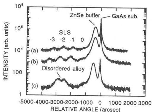
Fig.5 X-ray diffraction profile (a) for the as-grown  $\text{CdZnSe}/\text{ZnSe}$  SLS; (b) for the SLS annealed at 400 °C without the Si ion-implantation; and (c) for the Si implanted and annealed SLS (300 °C).
