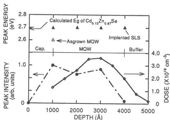
Fig.4 Depth profile of the peak intensity and peak energy of the 458.6 nm emission.
