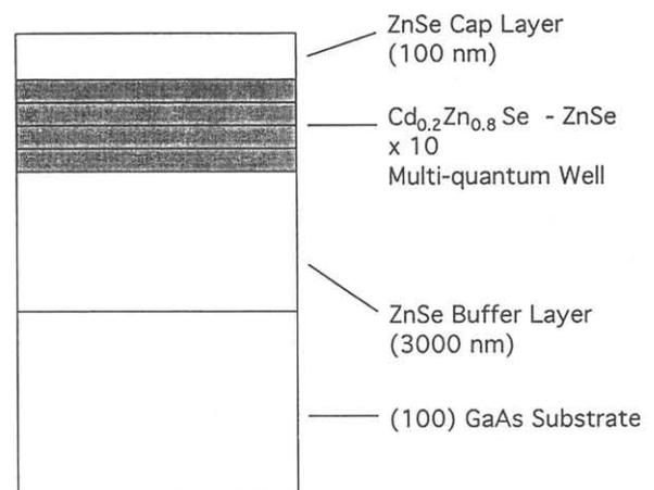
Fig.1 The structure used for the disordering experiments. The sample consisted of the following sequence of layers grown on a (100) GaAs substrate: (1) a ZnSe buffer layer (3  $\mu$ m), (2) a ten period superlattice of alternating 20 nm - Cd<sub>x</sub>Zn<sub>1-x</sub>Se ( $x=0.2$ ) and 10 nm - ZnSe layers, and (3) a ZnSe cap layer (0.1  $\mu$ m) to prevent degradation of the crystalline quality of the SLS during ion-implantation and annealing.
