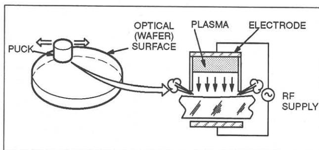
Fig. 1. Plasma assisted chemical etching (PACE).
