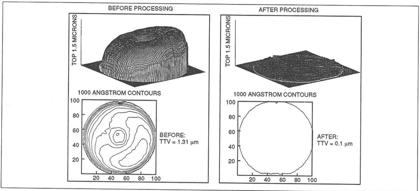
Fig. 5. 200 mm wafer flattening demonstration.
