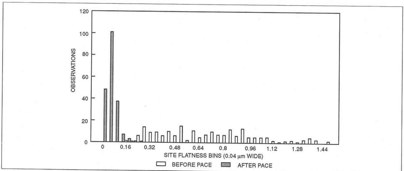
Fig. 6. TTV experiment: site flatness, before and after processing.
