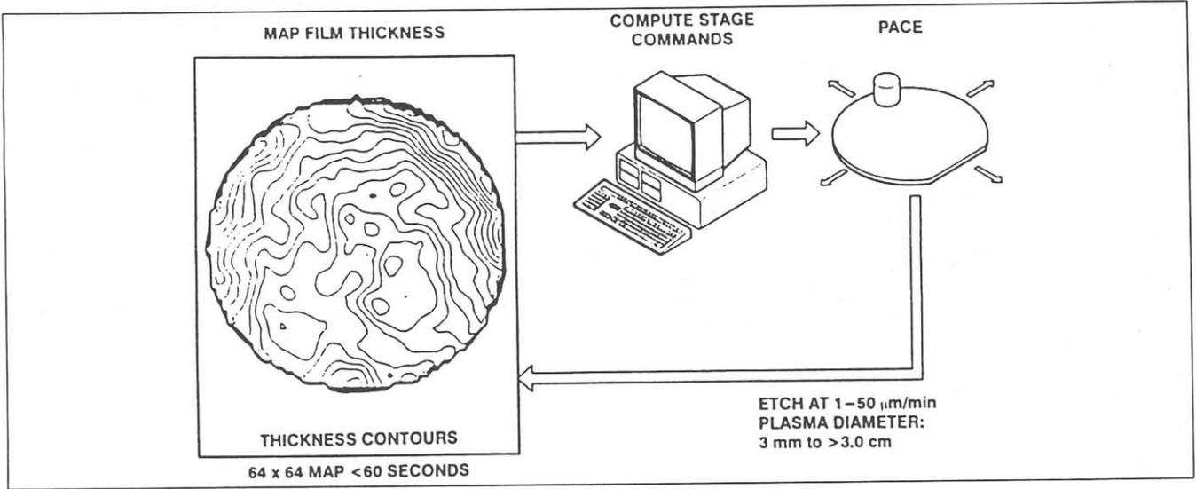
Fig. 2. SOI wafer thinning process.
