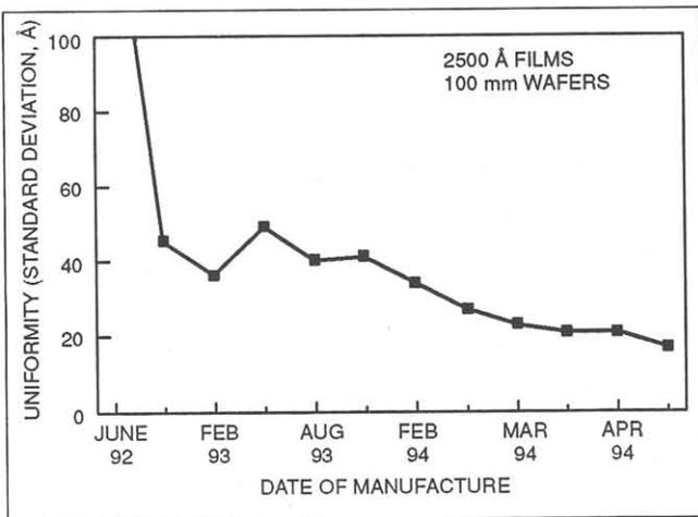
Fig. 4. SOI thickness uniformity: improvement June 1992 - April 1994.
