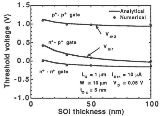
Fig. 3 Dependence of threshold voltage on SOI thickness.
