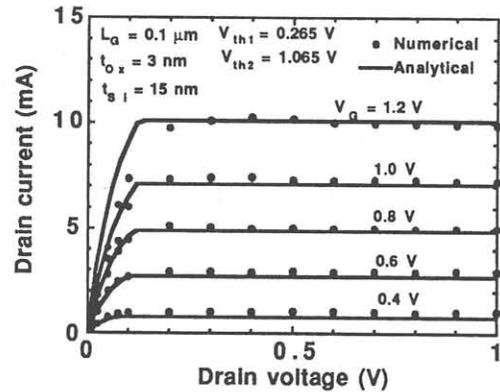
Fig. 6 Comparison between numerical and analytical current-voltage characteristics.
