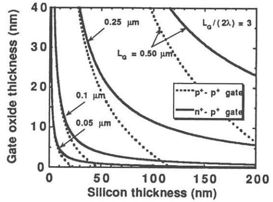
Fig. 5 Relationship between SOI and gate oxide thicknesses for various gate lengths.
