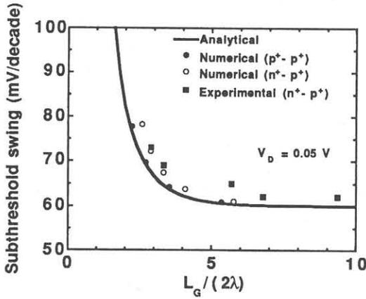
Fig. 4 Dependence of subthreshold swing on  $L_G/(2\lambda)$ . Device parameters used in numerical calculation:  $t_{Ox} = 5$  nm,  $L_G = 0.1$   $\mu\text{m}$ , and various  $t_{Si}$ . Experimental device parameters:  $t_{Ox} = 9$  nm,  $t_{Si} = 40$  nm, and various  $L_G$ .
