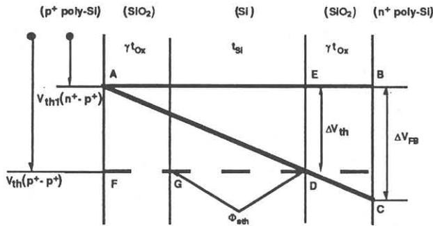
Fig. 2 Schematic potential distributions: a dashed line corresponds to a  $p^+ - p^+$  double-gate device and a solid line to a  $n^+ - p^+$  double-gate device.
