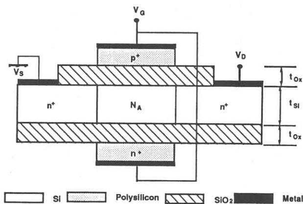
Fig. 1  $n^+ - p^+$  double-gate SOI MOSFET.
