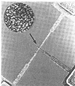
Fig. 1 Fabricated structure and an SEM photograph. The inset is the enlarged view of the active region, where the channel poly-Si and the gate cross.
