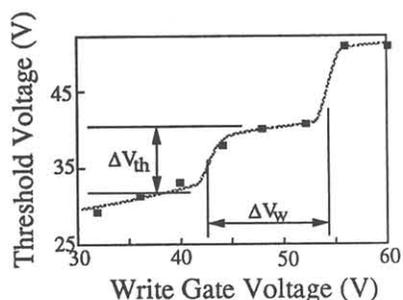
Fig. 3 The dependence of threshold voltage on write voltage.
