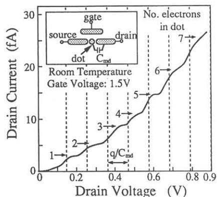
Fig. 7 A Coulomb staircase is evident when gate voltage is set slightly lower than the threshold voltage.
