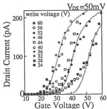
Fig. 2 Threshold quantization. The gate voltage is swept down from various write voltages.
