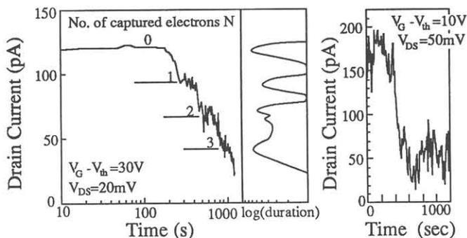
Fig.4 Temporal staircase and the integrated time for each current level (left). A giant leap is sometimes observed when  $V_G - V_{th}$  is smaller than the case shown on the left (right).
