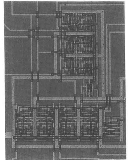
Fig. 5. Network configuration and photomicrograph of test vMOS neural network.
