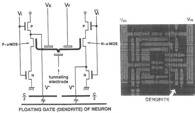
Fig. 2. Complementary vMOS differential source-follower circuit for synapse cell.
