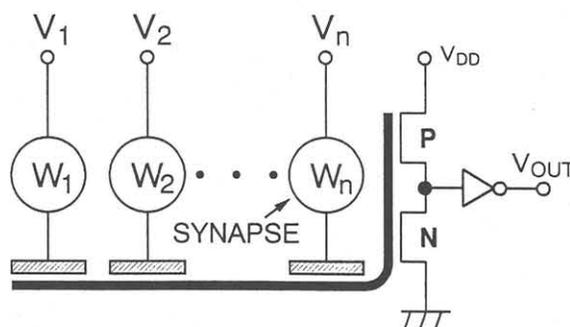
Fig. 1. Schematic of a neuron module composed of a complementary  $\nu$ MOS inverter and synapse cells.
