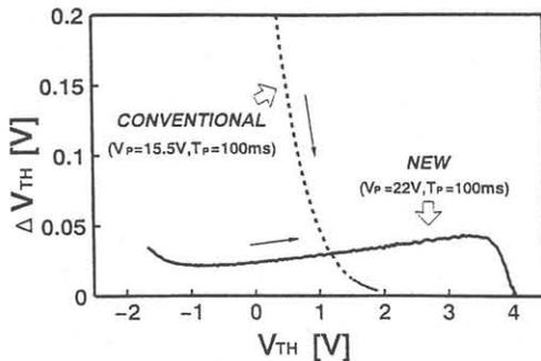
Fig. 8. Acceleration effect in the synapse cell.
