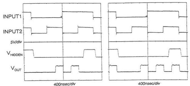
Fig. 6. Measured output characteristics of the test neural network which learned XOR and OR Boolean functions.
