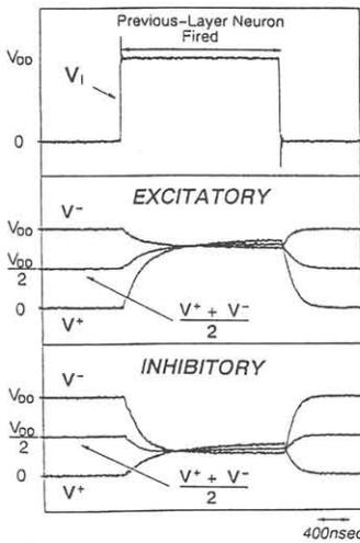
Fig. 3. Measured output wave forms of N-vMOS ( $V^+$ ) and P-vMOS ( $V^-$ ) source followers in the synapse cell.
