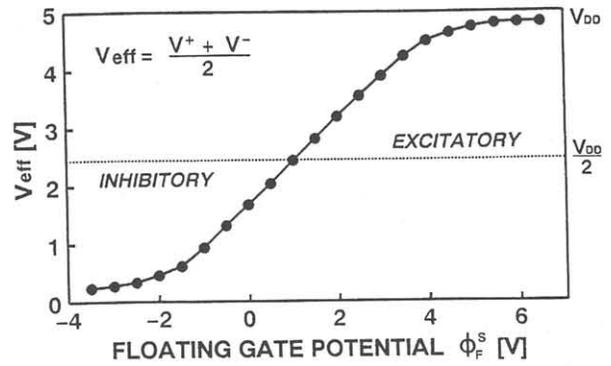
Fig. 4. Measured synapse output as a function of the synapse floating-gate potential.
