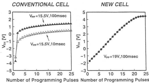
Fig. 7. Comparison of weight-updating characteristics of conventional cell (without source follower feedback) and new synapse cell (with feedback).
